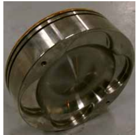
Piston top made of 42CrMo4 (Da=320mm)
