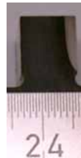
Electron beam hardened groove edge (hardness layer depth (ht) up to approx. 2mm)
