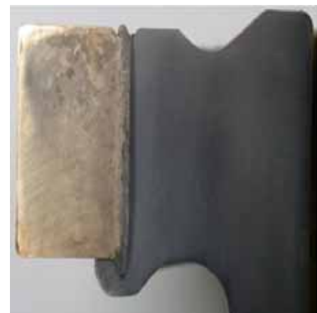
bronze-steel-compound weld depth: 25mm
