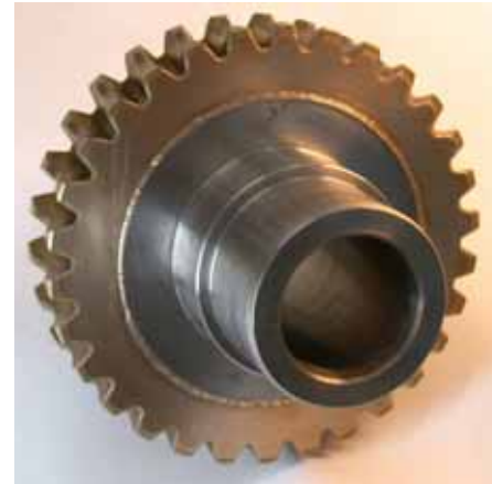
Electron beam welded worm wheel CuSn-St
