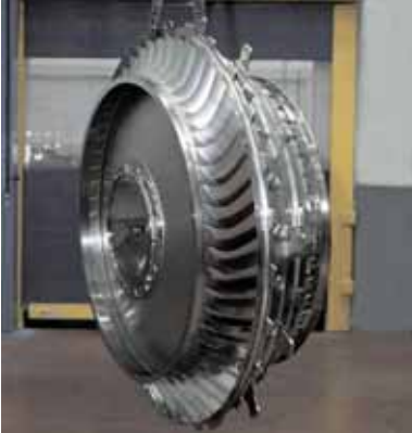
Pic 7: EB welded front bearing housing for Trent 700
