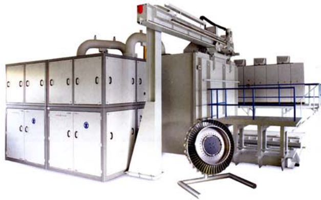
The welding is done in large vacuum chambers to prevent dispersion of the electron beam
