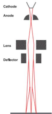
Figure 48: Multiple-beam process of three weld seams (left) schematic representation of a 3-beam process (right).
