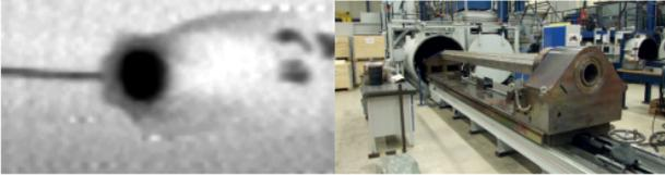
Figure 44: On the left the electron-optical image of a welding process clearly showing joint and keyhole, but also something of the flowing and solidification of the melt. On the right, a component is shown that can only be welded with ELO-Online.
