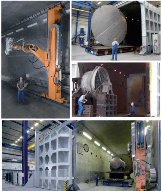
Figure 68: Large-chamber machine type K6000 (chamber volume 630 m<sup>3</sup>) with internal EB generator on the robot arm (left), EB welding aluminium panels for Ariane 5 (top right), repair of a guide vane carrier of a gas turbine, (centre), rotation fixture with copper vessel, (bottom).
