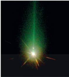
Figure 5: Effect of the beam: The workpiece heats up strongly, and X-rays are produced. Some electrons are scattered back and can be used for monitoring.
