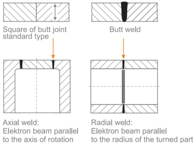
For the basic joint as shown in Figure 14 there are many options in the details, some of which can only be implemented with the beam welding process. The form of the joint
