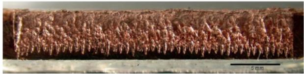
Figure 23: right: spiking when welding copper
