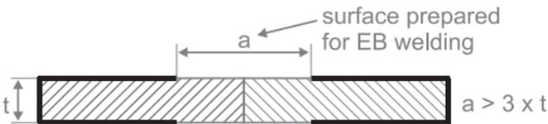
Figure 31: Recommended area of parts to be cleaned for electron beam welding.
