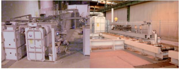
Figure 71: Schematic picture of a complete plant for producing EB-welded railway frog points.
