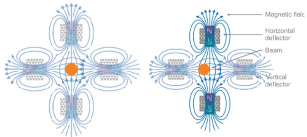
Figure 9: Deflection: In a homogeneous magnetic field perpendicular to the electron beam, the initially centred beam (left) is deflected sideways (right).
