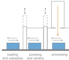
Figure 76: Load lock-type chamber machine, type S20.
