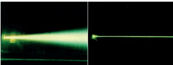
Figure 4: Beam expansion: An electron beam in a residual gas (500 mbar) shows beam expansion from multiple scattering (left); at 50 mbar, the expansion is almost absent (right).
