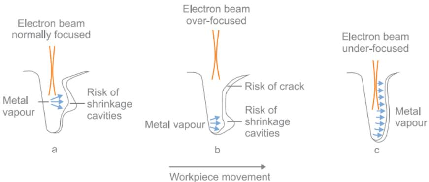
Figure 24: Model idea: relation between focus position and weld imperfections.
