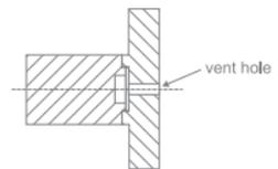
Figure 17: Component with vent hole.
