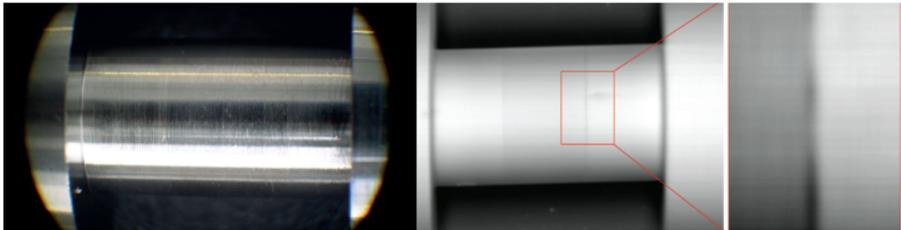
Figure 39: A component with a smooth machined surface where the joint gap is so narrow that it is not more evident than the traces of machining. In the electron-optical image on the right, the joint can be seen, because of the high contrasted imaging and also because of the different materials.
