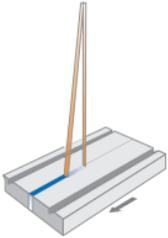
Figure 52: Weld and cosmetic seams with different focus positions.
