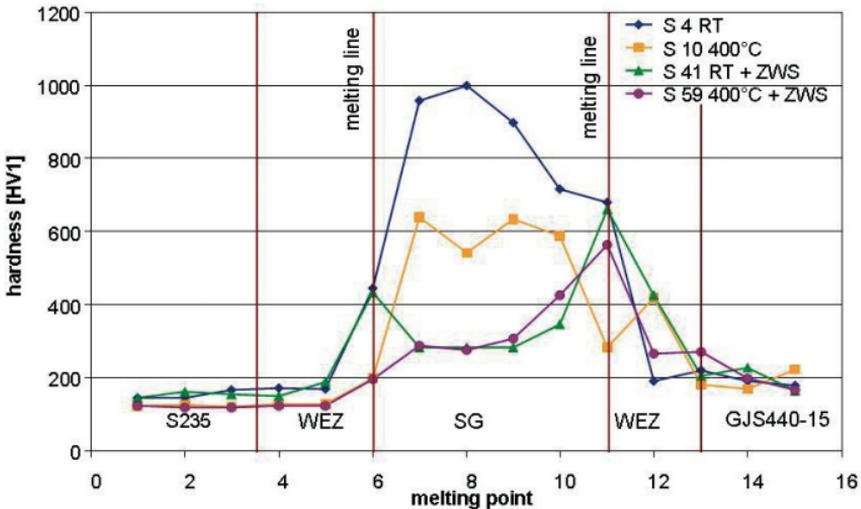
Figure 26: Comparison of hardness profiles in the joint zone in electron beam welding JS440 to S235.
