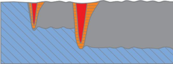
Figure 54: Preheating with an additional small weld pool.
