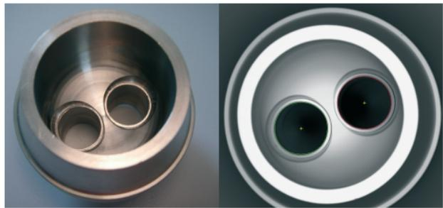
Figure 41: Photograph of a component (left) and its electron-optical image (right). The calculated centre points of the tubes are marked with small crosses.
