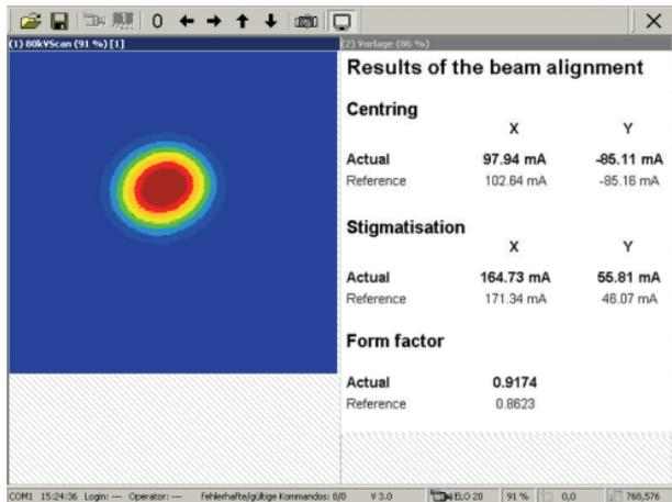
Figure 36: On the left of the results screen of the automatic beam alignment, the achieved beam profile is displayed in false colour. On the right a summary of the values found for the centring and stigmatising is shown, compared with the machine constants.
