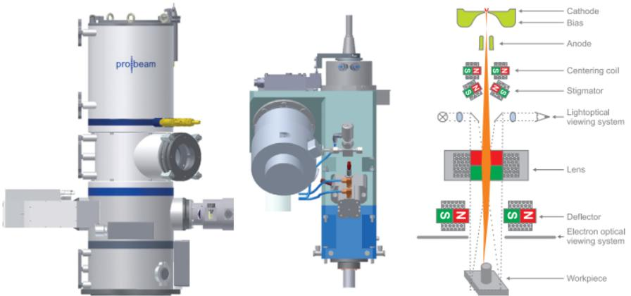
Figure 11: High-voltage column for high beam powers (left), low-voltage column for medium beam powers (centre), diagram of a beam column (right).
