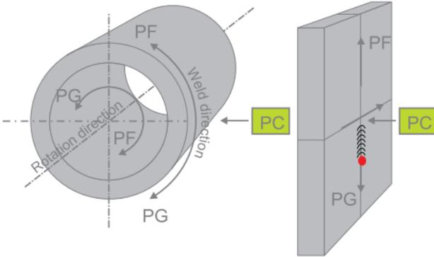
Figure 22: Diagram of the constrained positions PF and PG for cylindrical and flat parts.
