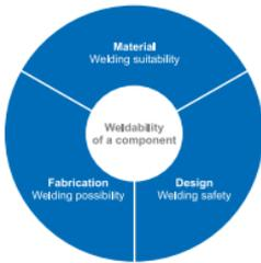
Figure 13: Factors that affect the weldability of a component according to DIN 8528-1.
