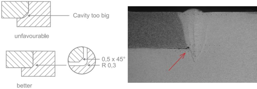
Figure 15: Left: Cavity permissible after processing. Right: Crack along the seam flank and to the weld root, starting from a cavity partly filled with melt
