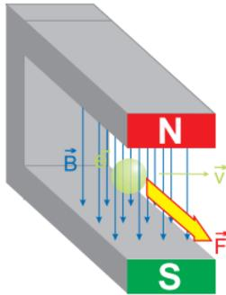
Figure 3: The Lorentz force  $\vec{F}$  acts on the electron in a magnetic field  $\vec{B}$  and is perpendicular to the direction of motion  $\vec{v}$  and to the field lines.
