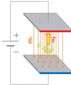
Figure 2: As a result of the Coulomb force  $\vec{F}$ , the electron in the electrical field  $\vec{E}$  experiences an acceleration in the direction of the anode.
