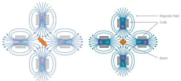
Figure 10: Beam shaping: With magnetic multipoles it is possible to correct astigmatism of the beam. The astigmatism (left) is corrected by magnetic fields (right).
