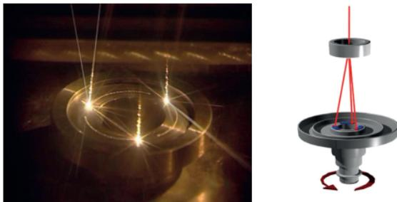
Figure 49: Welding an axial weld with three pools and moving beam (left). Model of welding an axial weld with three pools and moving workpiece (right).
