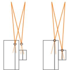
Figure 51: Radial welds with the 2-beam technique, left without and, right, with the dynamic lens.
