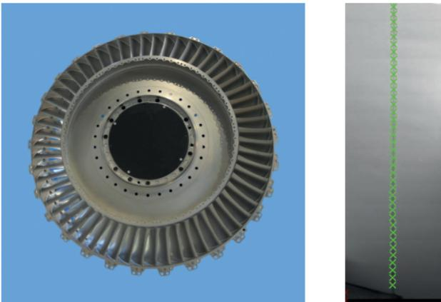
Figure 42: On the left a Ring-of-Vanes for aircraft turbines (diameter 1600 mm, Trent 900); on the right an electron-optical image of a joint between two vanes and its evaluation.
