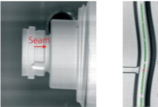
Figure 40: Electron-optical image of a pressure sensor for injection systems (left) and the details of its joint gap (right). The green and red crosses are reference points for automatic seam tracking.
