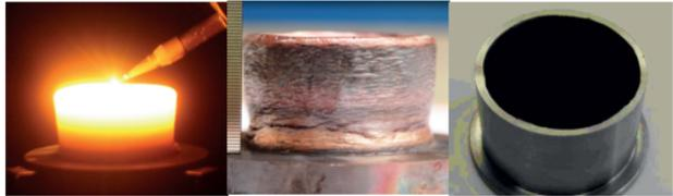
Figure 30: Sequence of steps for rapid prototyping of three-dimensional structures by means of an electron beam (surfacing) (left: building the structure; centre: resulting structure; right: structure after turning).
