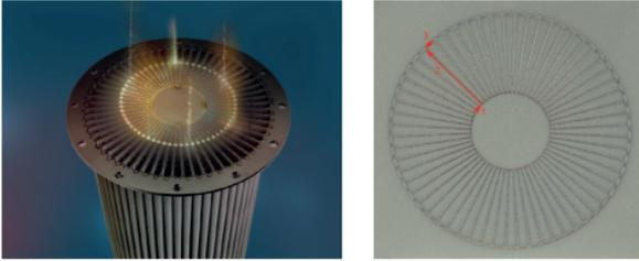
Figure 50: Welding with 60 beams on a soot filter (left). Welding sequence with 60 beams; example for one beam (right).
