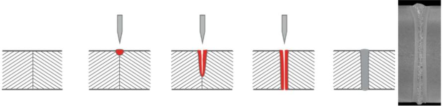
Figure 6: Deep-penetration effect: Melting and vaporising enable the beam to penetrate the material deeply. The weld pool penetrates the workpiece. Right: Micrograph of a full penetration weld in 50 mm thick steel, S355.
