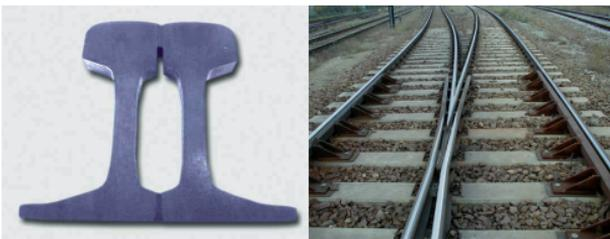
Figure 69: Section of a railway frog point welded with an electron beam.
