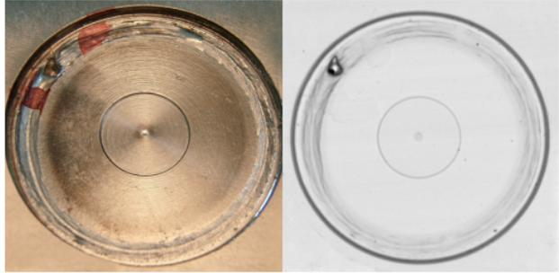
Figure 45: A photo of an axial weld with an open pore
