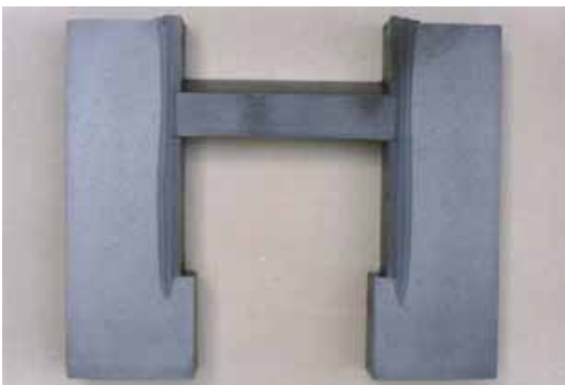
Figs. 190, 191: Section through the stator of a steam turbine. The welds are between 80 to 140 mm deep with a wall thickness of the cladding between 5 – 8 mm.
