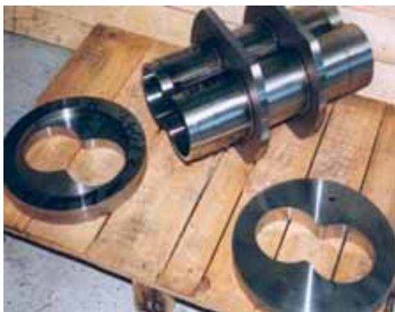
Figs. 168, 169: Housing of a twin-screw-extruder. Both, the longitudinal welds and the figure-of-eight profile welds were achieved with EB.
