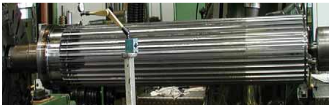
Fig. 25: 250 mm extension of a cog tube from 42 CrMo 4 V, weld depth 20 mm. A modification to an existing part.
