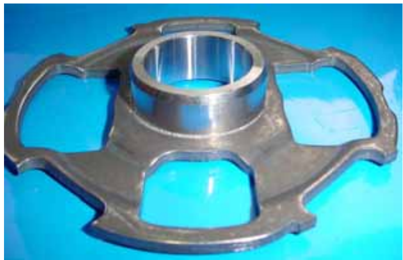
Fig. 17: Annealed sheet attached to a hub made from Ck 35.
