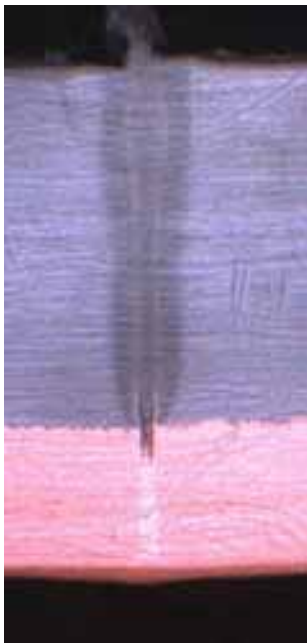
Fig. 119: Steel-copper composite with imperfections in the transition zone.
