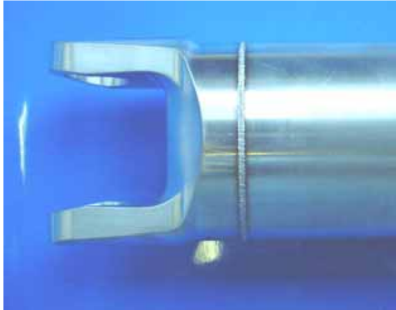
Fig. 55: Drive shaft, dia 80 mm, material AlMgSi 1.
