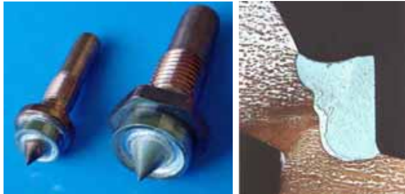
Figs. 127, 128: Brazing of copper to titanium with silver solder.
