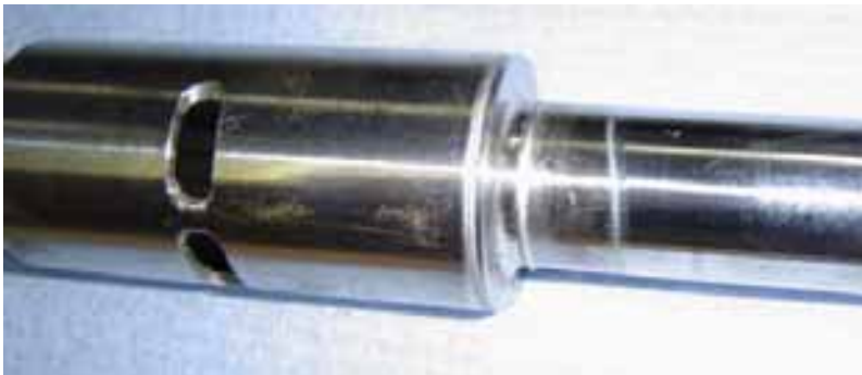
Fig. 163: Piston rod of a shock absorber, EB welded from two tubes and an intermediate disc.
