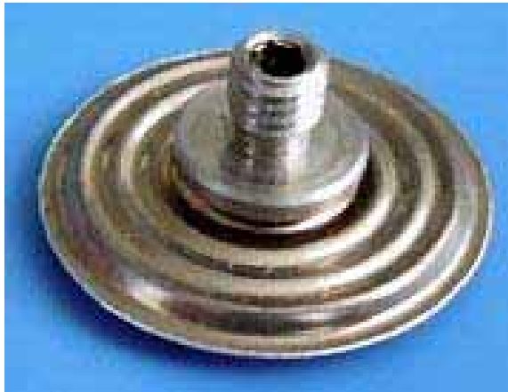
Figs. 216, 217: 20 \mu\text{m} thin rupture membranes or metering diaphragms are EB welded. Figs. 218, 219: Preformed thin sheets are welded to produce pressure cells or bellows.
