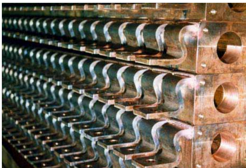
Fig. 75: High-current conductors with internal cooling used for a tinning plant.
