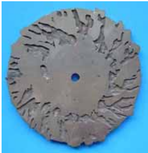
Fig. 40: Tubular porosity in welded GGG 60.
