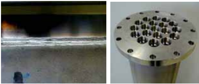
Fig. 36,37: Circumferential weld and top view of a filter module.
