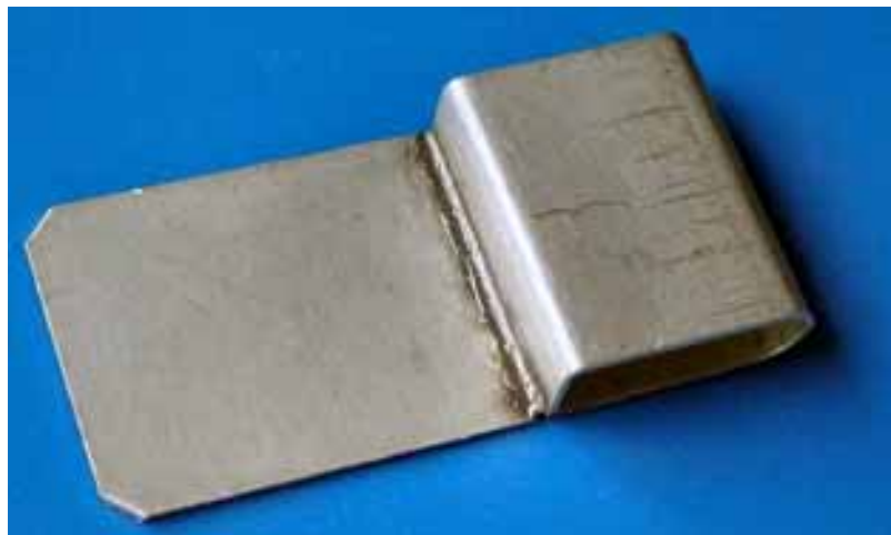
Fig. 56: Microweld in 0.7 mm thick aluminium sheet.
