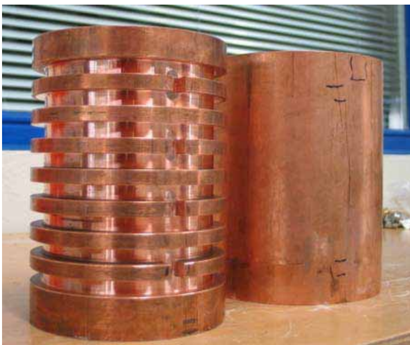
Figs. 65, 66: Cooler fabricated from a profiled body and outer sleeve; welded on the end faces.
