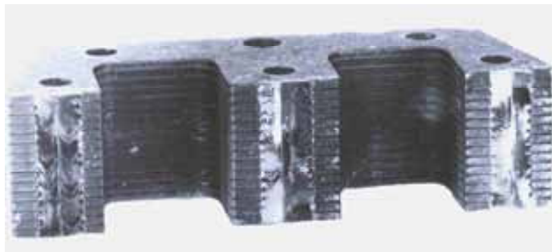
Fig. 43: Transformer laminates of silicon iron.
