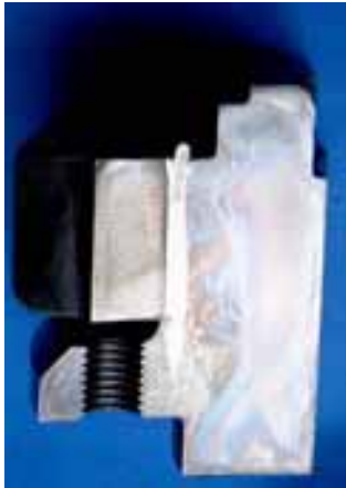
Fig. 23: cross section of a gear made from 21 NiCrMo 2.
