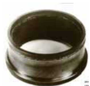
Fig. 126: Punching tool with steel body and hard metal ring.
