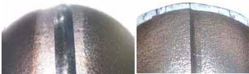
Fig. 89: Upper bead and weld root of a reaction chamber.
