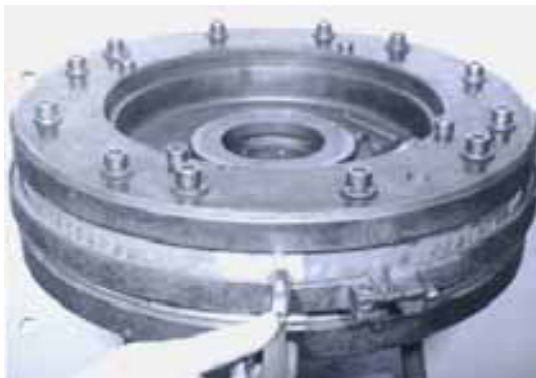
Figs. 269 to 272: upper left – lower half of welding jig, upper right – blades located using a “blade punch”, lower left – complete welding jig with stator in place, lower right – profiles of welded vanes.
