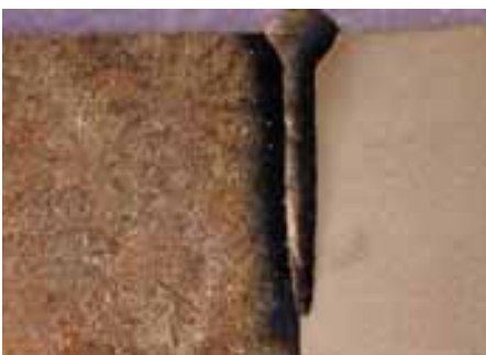
Figs. 114, 115, 116: Even steel to stellite (left) or copper to aluminium (centre and right) can be welded
