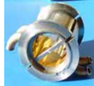
Fig. 133: Infrared cavity. The inner gold plating must not be overheated or coated with vapour. This has been achieved by reducing the wall thickness in the weld area.
