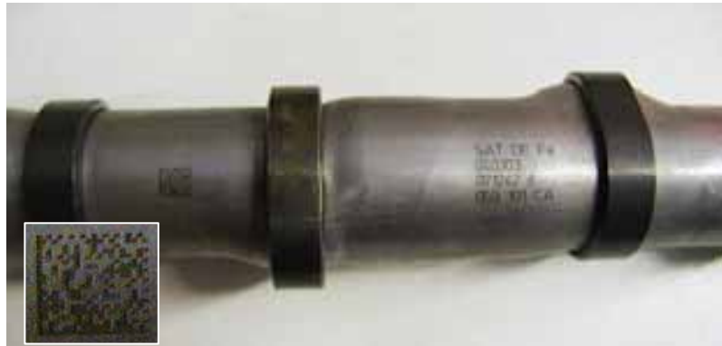
Fig. 274: Camshaft are supplied with engraved data matrix code and plain text.
