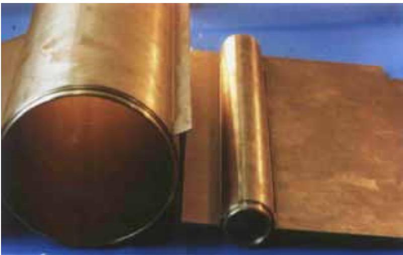
Figs. 151, 152, 153: Tolerance rings exactly ground to size are welded from both sides, whereas the centre remains un-welded to maintain dimension.
