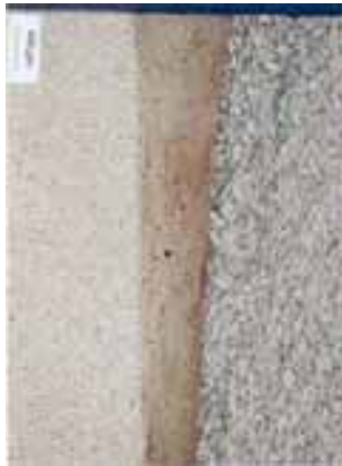
Fig. 61: Section through a forged rim of AZ 80 and a cover of ZK 60.
