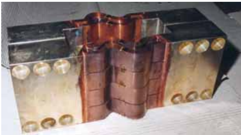
Fig. 71: High current flexible conductors for power distribution, fabricated from multiple copper laminates welded to silver coated connections.
