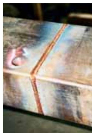
Fig. 76: Detail of Fig. 75. Radial weld of a box section, 15 to 40 mm weld depth, CNC controlled.
