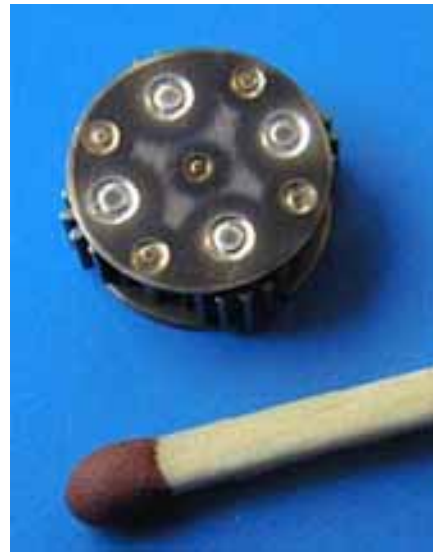
Figs. 233, 234: Pinion and planetary gear of a hand-prosthesis with 17 EB welds.
