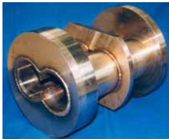
Figs. 168, 169: Housing of a twin-screw-extruder. Both, the longitudinal welds and the figure-of-eight profile welds were achieved with EB.
