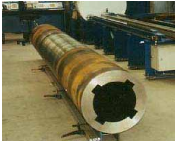
Figs. 210, 211: Spindles of large milling machines with internally machined profiles.
