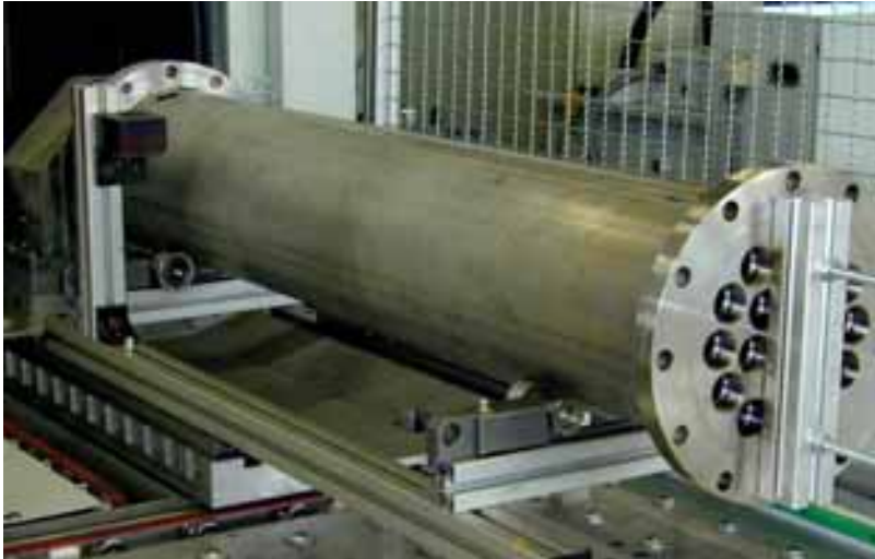
Fig. 35: Filter-module made from stainless steel.
