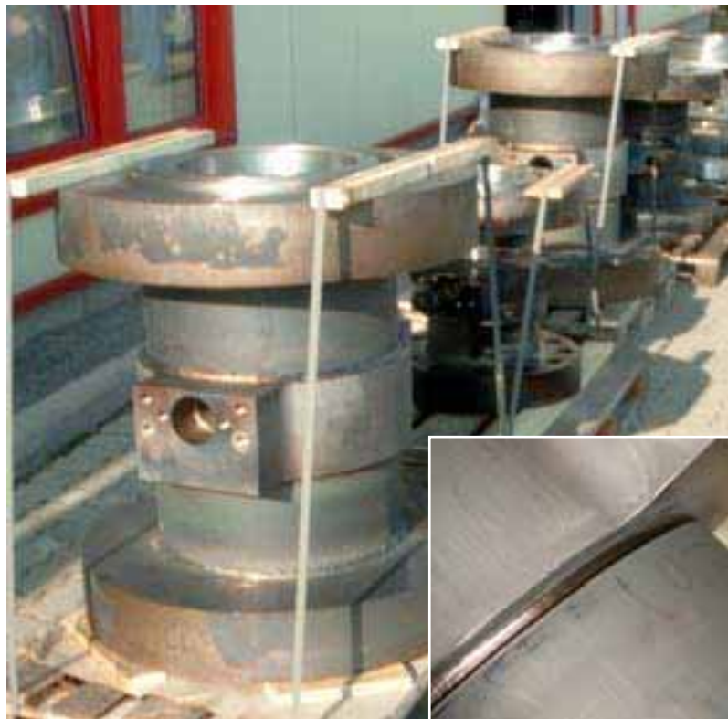
Figs. 33,34: High-pressure valves made from hot-working steel.
