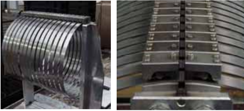
Figs. 151, 152, 153: Tolerance rings exactly ground to size are welded from both sides, whereas the centre remains un-welded to maintain dimension.
