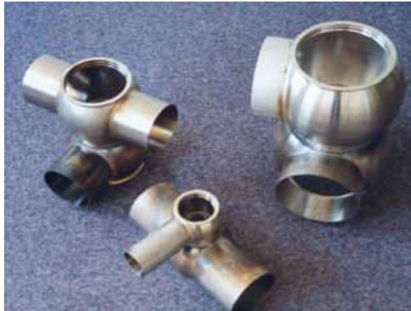
Fig. 31: Valve combinations for the drinks industry. For hygienic reasons, corrosion resistant, smooth seams without undercuts are absolute requirements.
