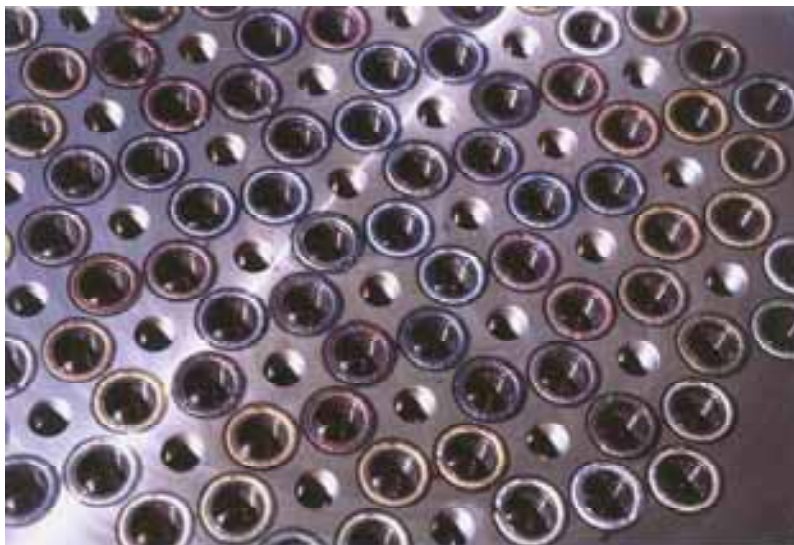
Fig. 82: More than 400 nozzles made of Inconel 718 or X5 Cr Ni Nb 18 10 are welded into the injection plate of the Ariane rocket.
