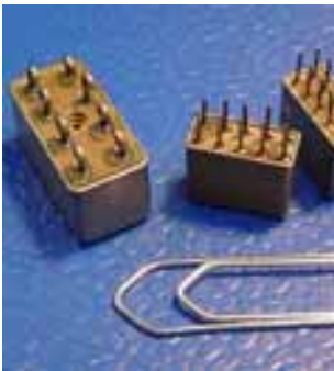
Fig. 232: Relay enclosure with heat sensitive glass feed-through.
