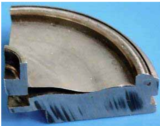
Figs. 212, 213, 214, 15: Welding of thin diaphragms for various applications is possible with electron beam welding.
