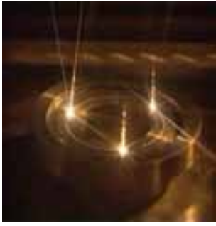
Fig. 157: Triple beam welding technique.
