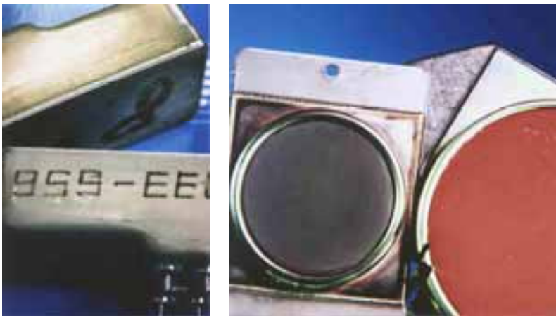
Figs. 134., 135: Left - encapsulated pacemaker, right - data logger.
