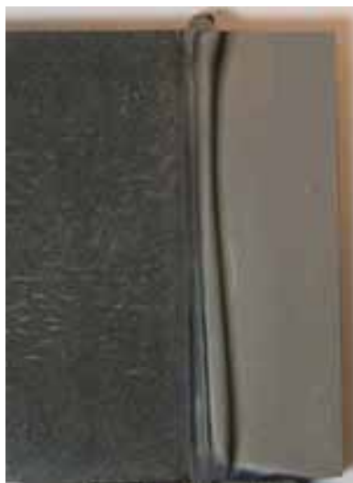
Fig. 102: St 37 welded to X2 Ni Co Mo 18 9 5, 100 mm thick.
