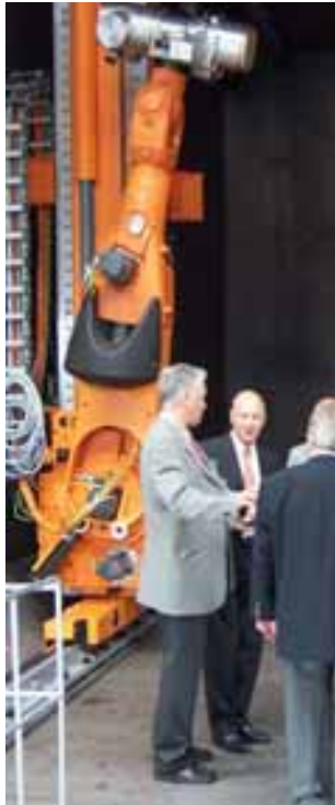
Fig. 8: Gantry traverse (12 x 6 m) mobile electron beam gun, mounted on a 3 m robot arm.
