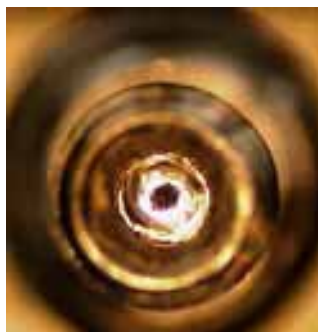
Figs. 226, 227: Screw thread EB welded from the front side.
