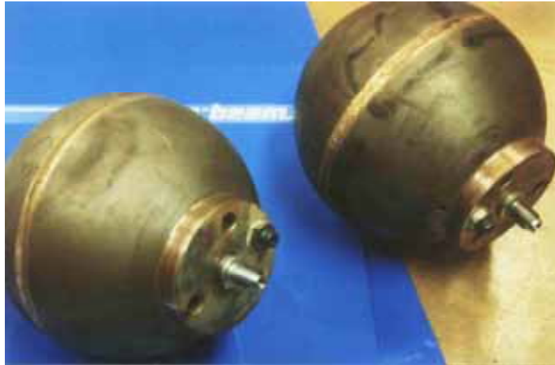
Fig. 77: Copper radiation absorber used in a solar power plant. Parabolic reflectors and a heat pipe produce super-heated steam to power a turbine.
