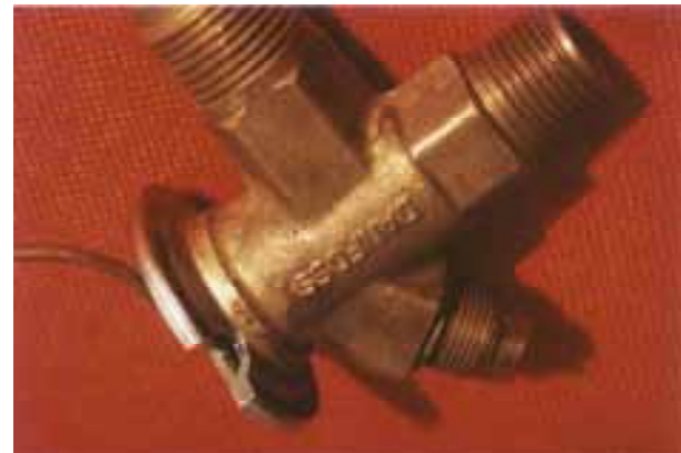
Figs. 212, 213, 214, 15: Welding of thin diaphragms for various applications is possible with electron beam welding.
