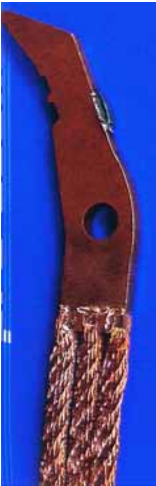
Fig. 141: Cold strain-hardened copper must not lose its hardness when welding four joints.
