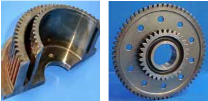
Fig. 176: Gear combination fabricated of two thin discs.
