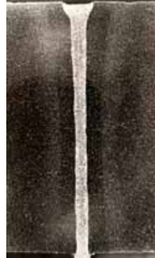
Fig. 27: Deep penetration weld in X5 CrNi 18 9, 1 mm wide, 25 mm deep with only 2.7 kW beam power.
