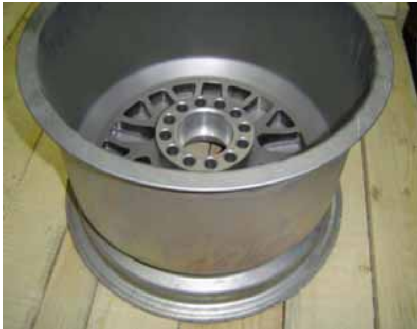
Fig. 62: Rim of a racing car wheel made of AZ 80, radial weld 25 mm deep.
