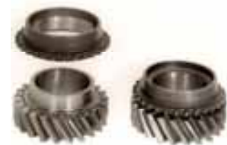
Fig. 6: Synchronesh gear from 1964.
