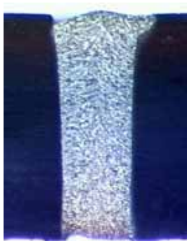
Fig. 29: Longitudinal tube weld in duplex steel, 7mm wide, and 22 mm deep. Beam power 15 kW.
