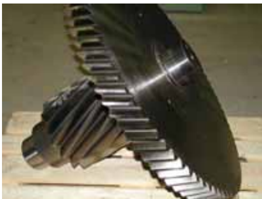
Figs. 160, 161: EB welding of all gears sizes is now accepted world-wide as the most frequent application for electron beam welding, mainly due to low distortion.
