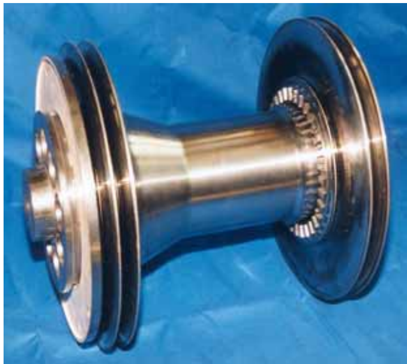
Fig. 24: clutch spindle torsionally stiff but flexible for bending- Materials 31 CrMoV 9 or 30 CrNiMo 8.
