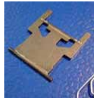
Fig. 228: Locking cam with four EB welds
