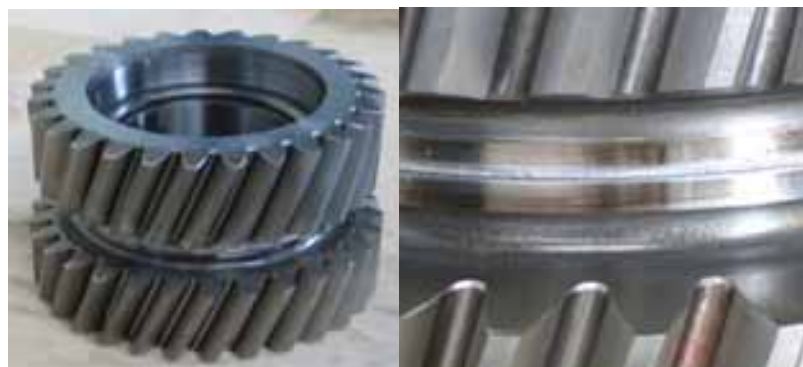
Fig. 20, 21: Twin gear made from 17 CrNi Mo 6, weld depth 9 mm.
