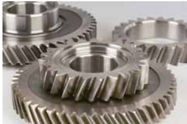
Figs. 160, 161: EB welding of all gears sizes is now accepted world-wide as the most frequent application for electron beam welding, mainly due to low distortion.
