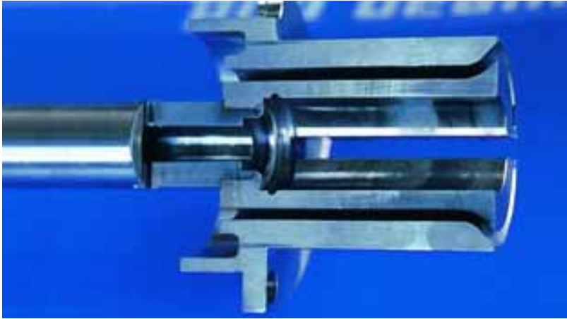
Fig. 178: A further development of the principle used in Figs. 167 and 177 is the introduction of curved shapes. Additionally a flange and a tube have been added.
