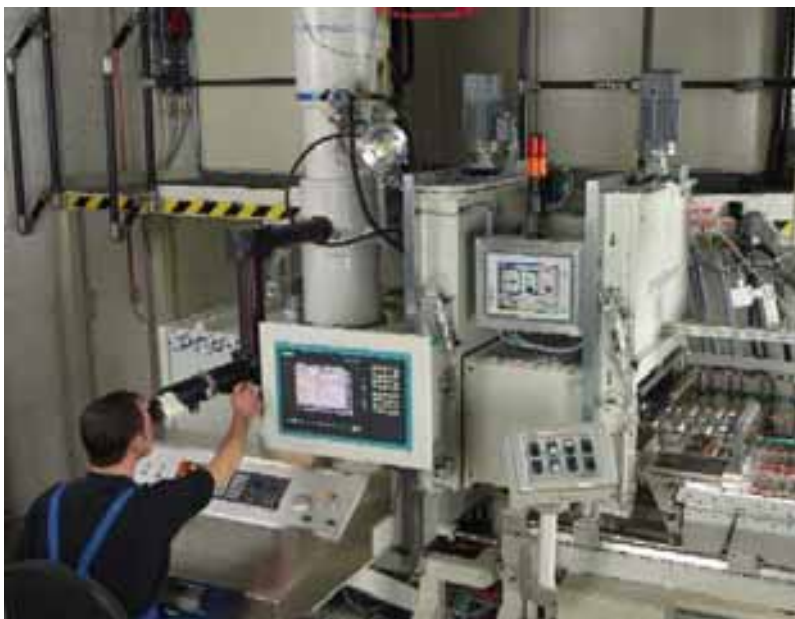
Fig. 7: Load-lock shuttle machine with 0.6 m 3 vacuum chamber. Automated, rapid exchange of work pieces transferred through the open lock-door (right).
