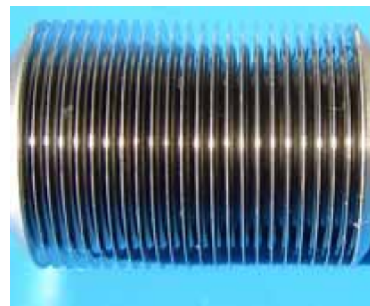
Figs. 216, 217: 20 \mu\text{m} thin rupture membranes or metering diaphragms are EB welded. Figs. 218, 219: Preformed thin sheets are welded to produce pressure cells or bellows.
