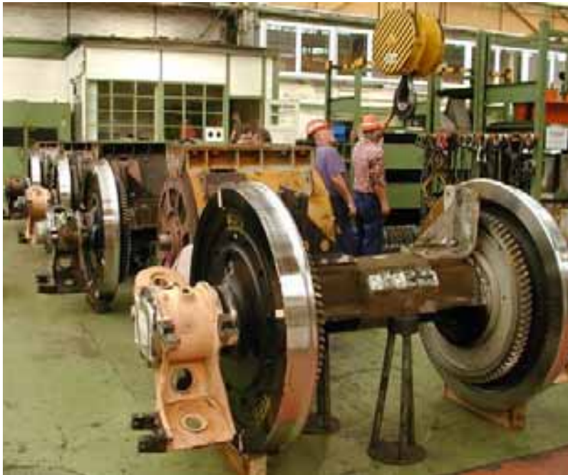
Figs. 263, 264: Assembled and installed after refitting the quill-bearing box.
