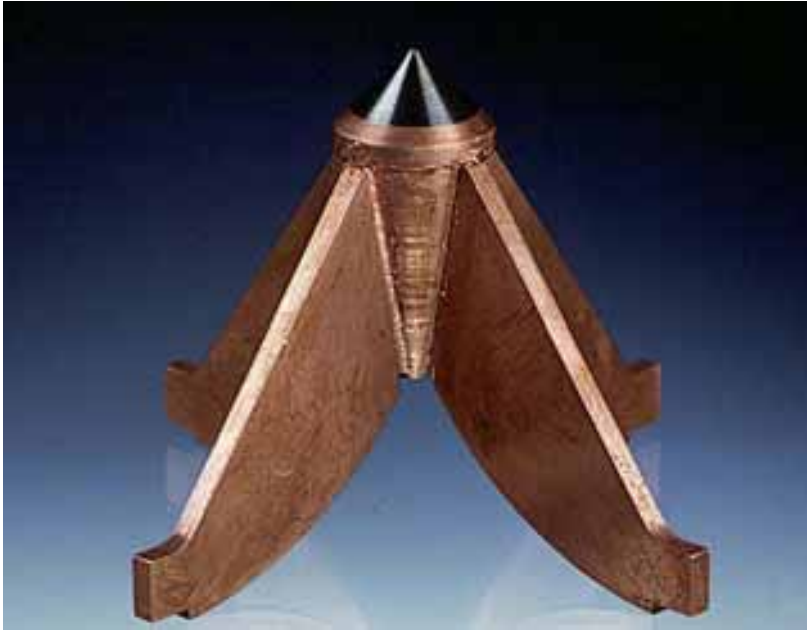
Fig. 170: High current cathode fabricated from a copper casting with integral tungsten tip and EB welded to four legs stamped from copper plate.
