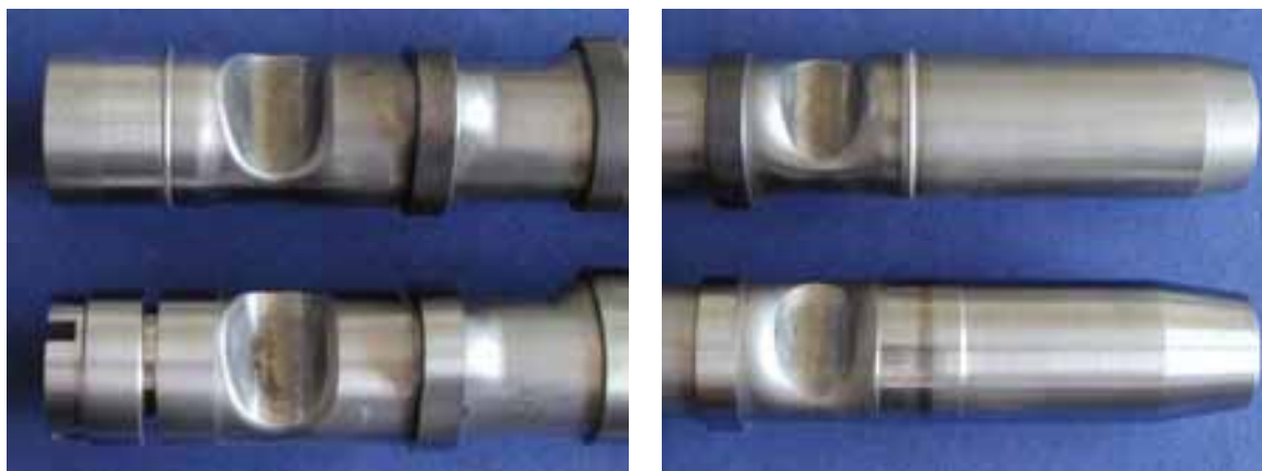
Figs. 279, 280: Camshafts after welding (top) and finish ground (bottom)
