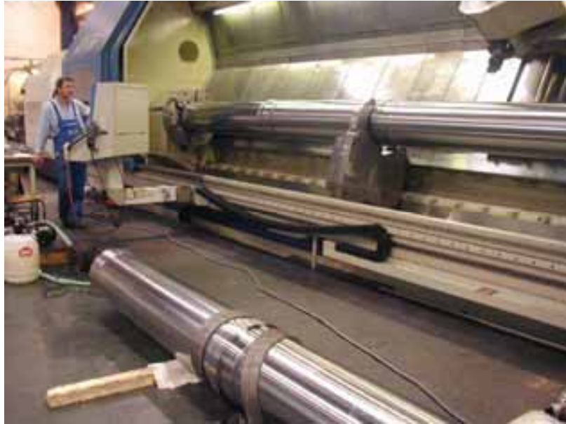
Fig. 240: Long piston rods fabricated by EB welding tube segments.
