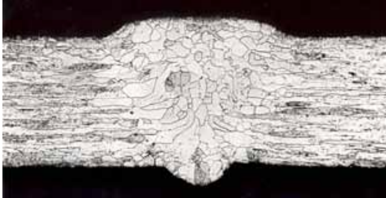
Fig. 26: Micro-weld of X 22 CrNi 17, 0.5 mm thick with only 100 W beam power (note the coarse grain structure).
