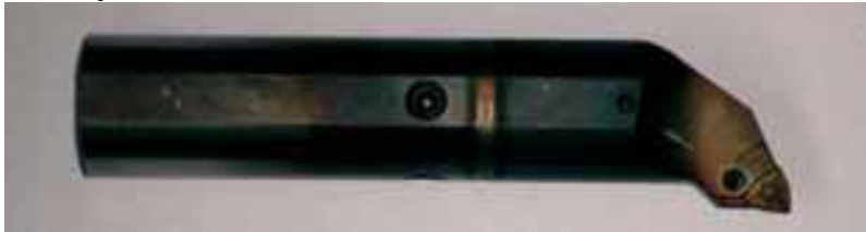
Fig. 18: Standard cutting tool with extension bar from 16 MnCr 5. Weld depth 20 mm.
