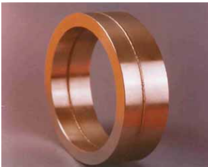
Figs. 63, 64: Section through SE-copper ring. Weld depth 35 mm.
