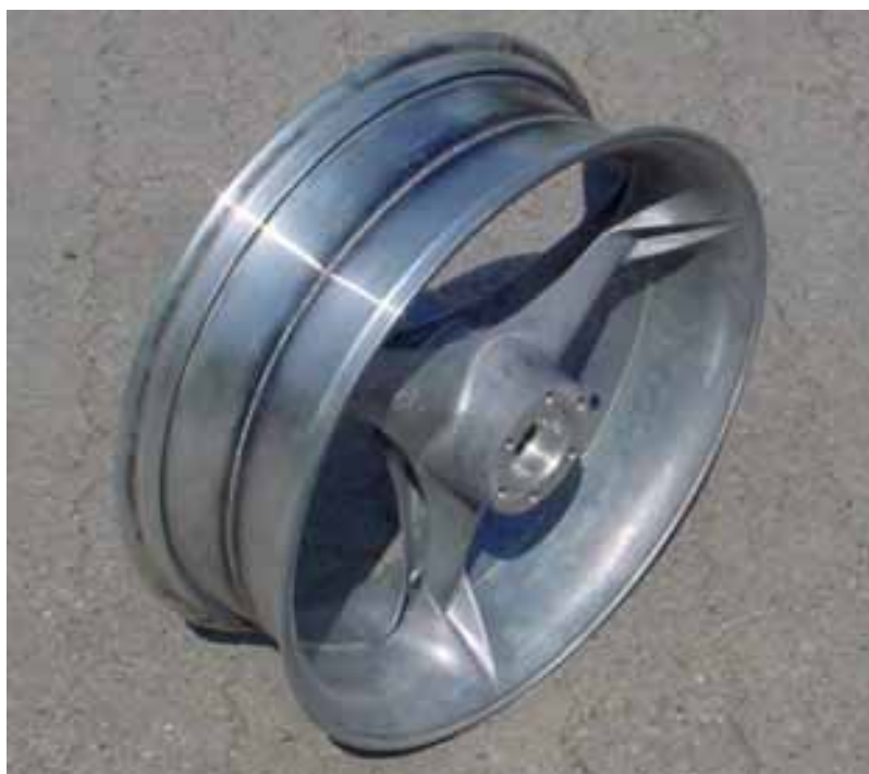
Fig. 53: Rim of a motorbike wheel made from pressure cast aluminium.
