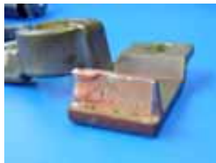
Fig. 129: Brass-copper joint with silver solder. The size of the fracture surface is used for quality control.
