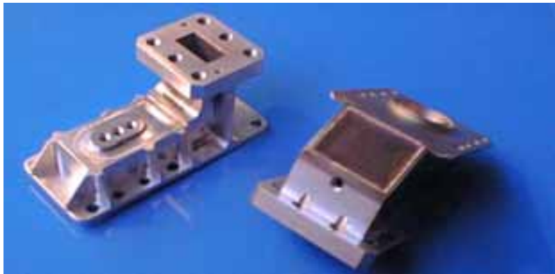
Fig. 202: Access opening for internal machining that are sealed by EB welding.
