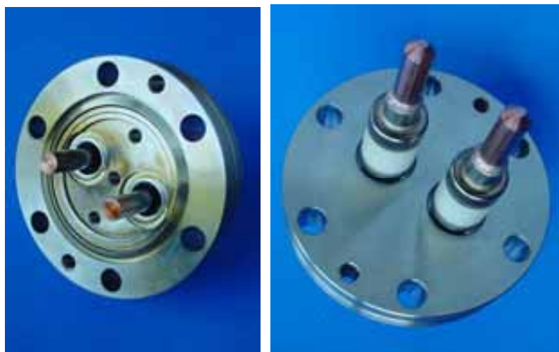
Figs. 142, 143: In order to avoid cracks due to the different thermal expansion between insulator and metal, the welds must be undertaken with minimum heat input.
