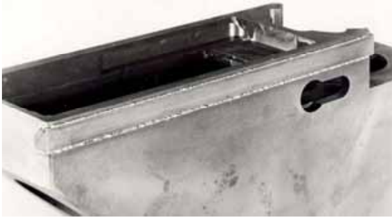
Fig. 111: Guide rail made of case hardening steel, welded with a nickel filler foil to cast iron.
