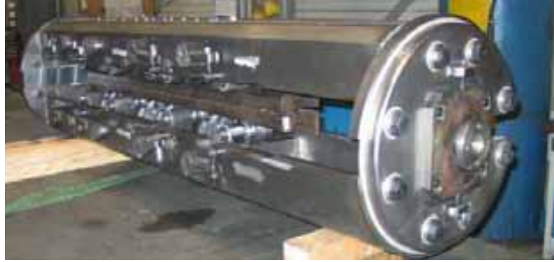
Fig. 14: Clamping fixture made from St 52.3.
