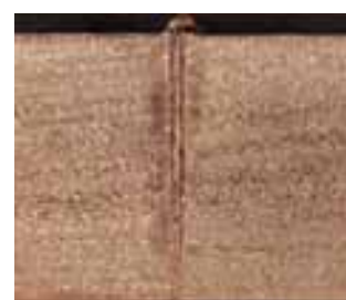
Figs. 63, 64: Section through SE-copper ring. Weld depth 35 mm.
