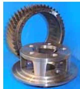
Figs. 155, 156: Pinion cage and driving gear fabricated with radial EB welds.
