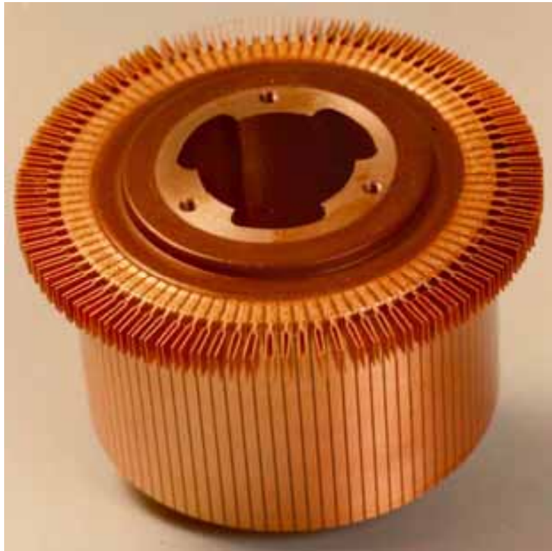
Fig. 140: Commutators of electric motors with 8 mm deep welds (pulsed operation) very close to temperature sensitive insulation.
