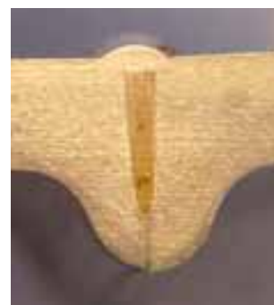
Fig. 54: Cross-section of the rim on which a cosmetic pass can be seen.
