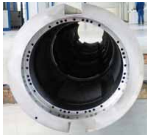
Figs. 210, 211: Spindles of large milling machines with internally machined profiles.
