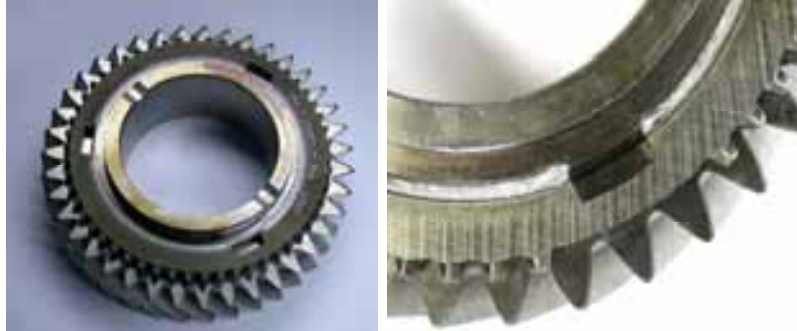
Figs. 158, 159: Indexing gear, EB welded with triple beam technique.
