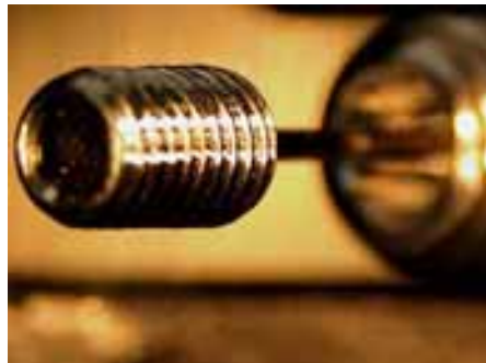
Figs. 226, 227: Screw thread EB welded from the front side.
