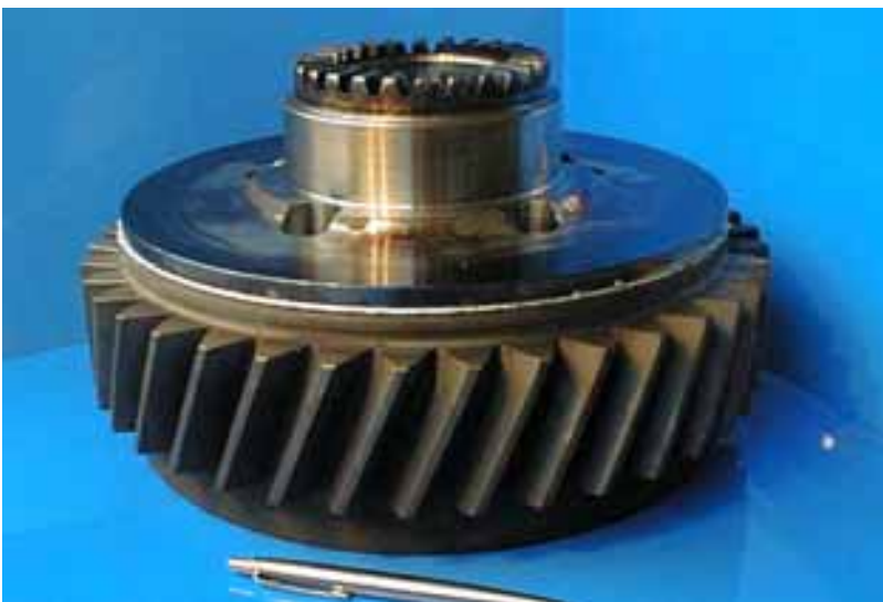
Figs. 155, 156: Pinion cage and driving gear fabricated with radial EB welds.
