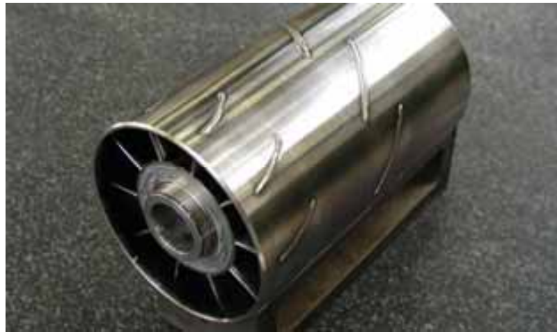
Figs. 206, 207: A large variety of designs become possible by using stake welds.
