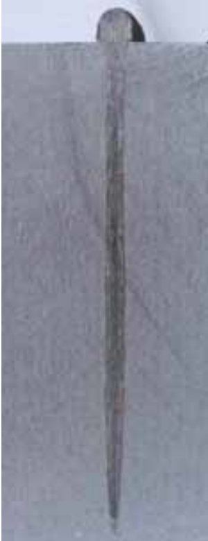
Fig. 32: A narrow, 45 mm deep weld seam in austenitic steel.
