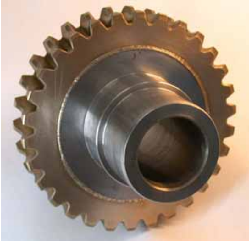
Figs. 188, 189: Bronze with good tribology properties is EB welded to low cost steel.
