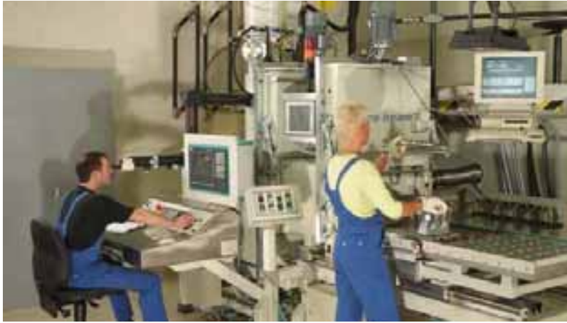
Fig. 277: Mounting and welding on a load-lock-shuttle machine.
