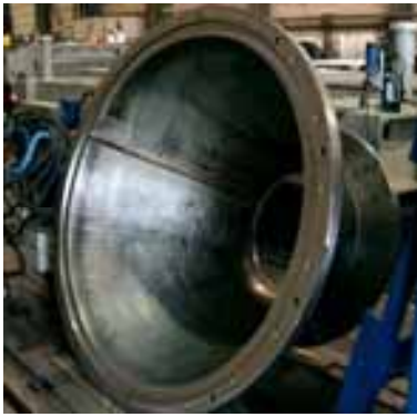
Fig. 244, 245, 246: Furnace parts - EB welded in a 20 m 3 chamber - used for the destruction of old ammunitions.
