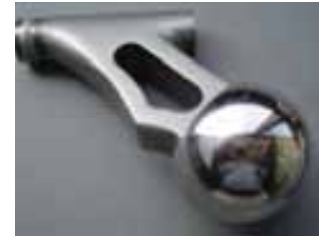
Fig. 5: EB welded hip prosthesis from 1963.
