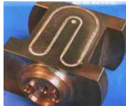
Figs. 208, 209: Any free programmable contour may be milled in the body and sealed by lid attachments.
