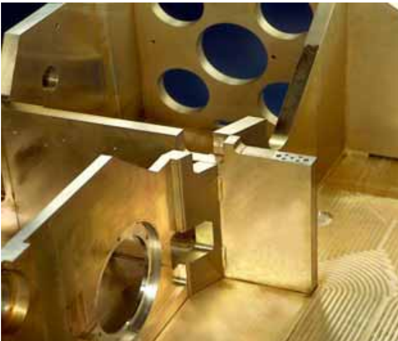
Fig. 164: Microscope frame fabricated from aluminium plates rather than machining from solid.
