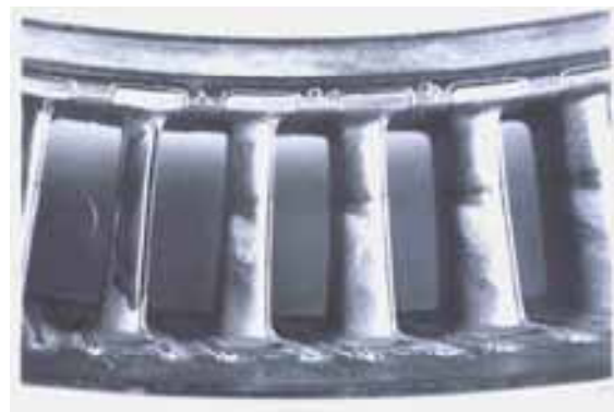
Figs. 269 to 272: upper left – lower half of welding jig, upper right – blades located using a “blade punch”, lower left – complete welding jig with stator in place, lower right – profiles of welded vanes.
