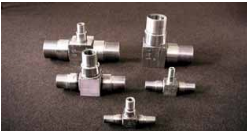
Fig. 38: High-pressure fittings from X6 CrNiMoTi 17 12 2, weld depth 15-26 mm.
