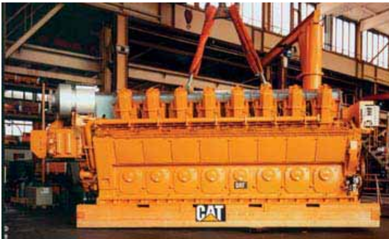
Fig. 247: EB welded "lifting lugs" for lifting marine engines weighing up to 140 ton.
