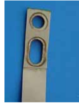
Fig. 224: Tension band, 30 \mu\text{m} thin, welded to an end terminal 70 \mu\text{m} thick.
