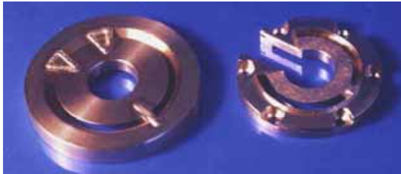
Fig 167: Complicated construction fabricated from inner and outer rings and ring segments; all manufactured from turned parts. Left – completed fabrication, right - finish machined part.
