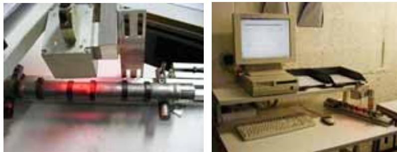
Figs. 275, 276: A laser scanner determines identifies each shaft on each workstation before processing.
