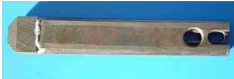
Fig. 187: A weaver's shuttle with internal grippers.
