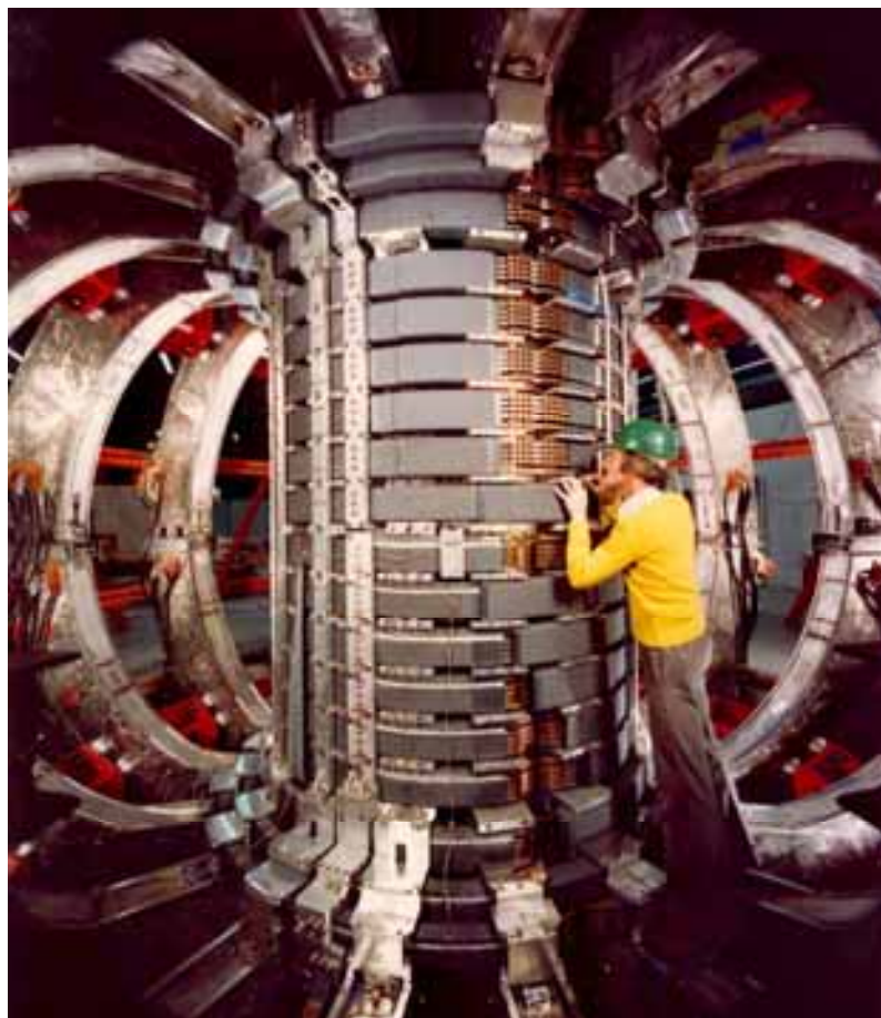
Figs. 69, 70: There are more than 1000 EB welded clamps of Cu Be 2 in the ASDEX fusion reactor.
