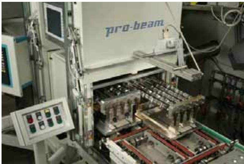
Fig. 278: Automated exchange of the 5-spindle work piece fixtures.
