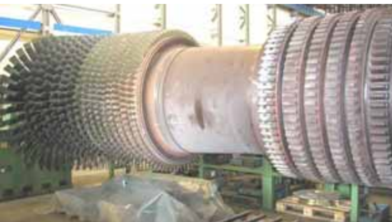
Fig. 258: Rotor of a gas turbine with a weight of 52 ton.
