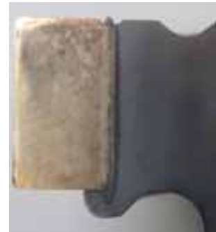
Figs. 188, 189: Bronze with good tribology properties is EB welded to low cost steel.
