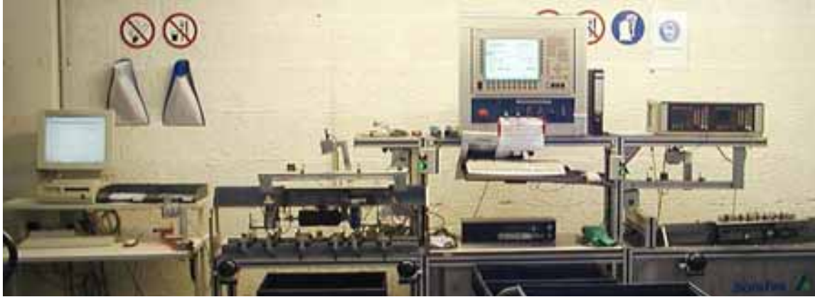
Fig. 281: Checking for run-out after welding and data protocol production.
