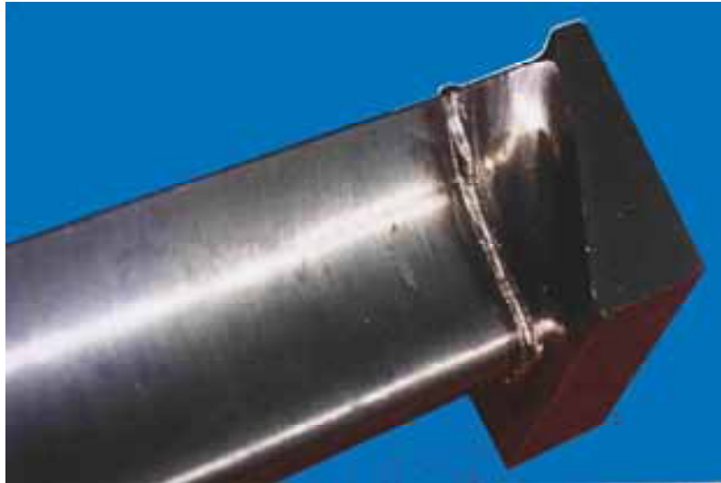
Fig. 192: 3D profile weld of a steam turbine vane, welded with simultaneous focus, beam current and welding speed control.
