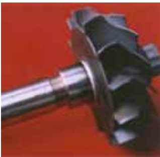
Fig. 106: Turbocharger fabricated from a free cutting steel shaft and an Inconel impeller.
