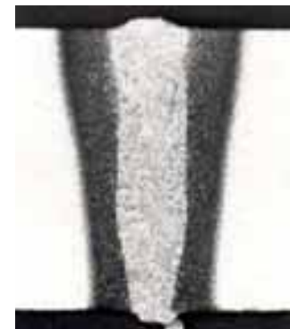
Fig. 22: Macro section 25 CrMo4, weld depth 3 mm.
