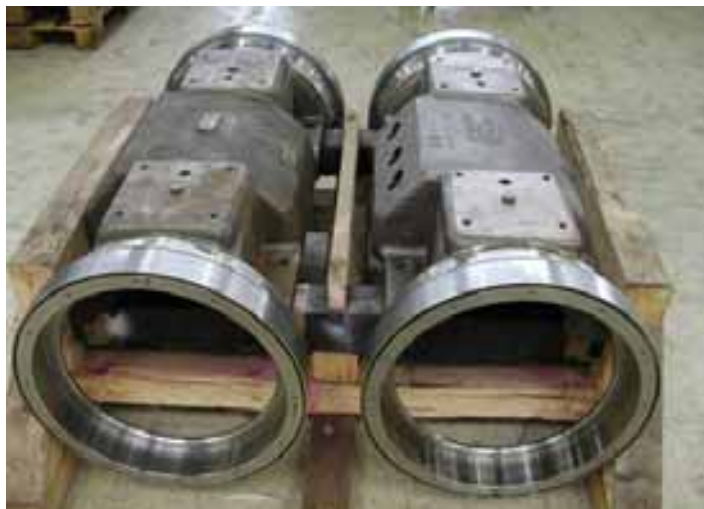
Figs: 259 – 261: Repair of quill bearing boxes for locomotives.
