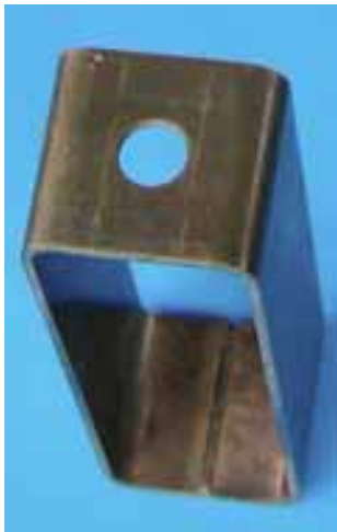
Figs. 69, 70: There are more than 1000 EB welded clamps of Cu Be 2 in the ASDEX fusion reactor.
