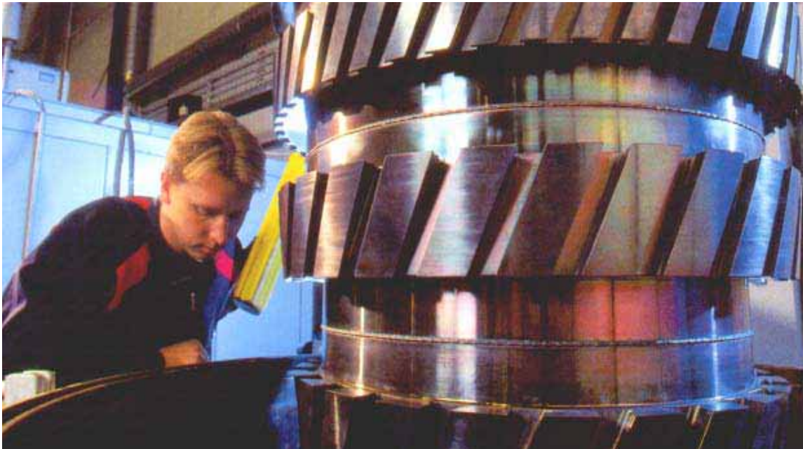
Fig. 237: Turbine shaft of a power plant. The individual segments can be machined on smaller machines.
