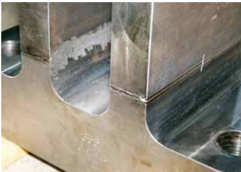
Fig. 249: Welding seam on lifting lug, right - as welded, left - after grinding and x-ray
