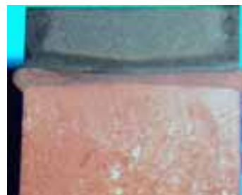
Figs. 112, 113: Nozzles welded of copper because of its good heat conductivity and steel for its wear resistance, are used in injection-moulding machines. The central bore is drilled after welding.
