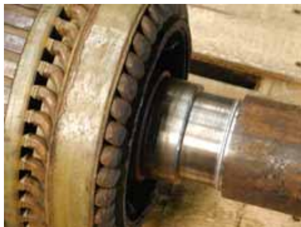
Figs. 251, 252: A worn out valve body of 42 CrMo 4 was reconditioned by inserting a new sleeve. Weld depth 55 mm.
