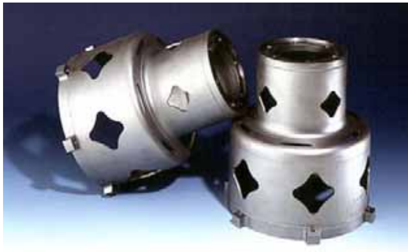
Fig. 166: Hollow shafts fabricated from laser cut drawn tubes and end flanges – two radial and one axial EB welds.
