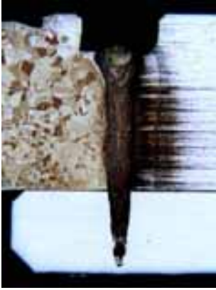
Fig. 229: Macro of a sensor weld 0,2 mm wide.
