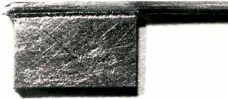
Fig. 98: Tungsten "Flag", wire diameter and flag thickness 0,5 mm, welded with pulsed electron beam.
