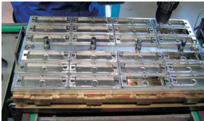
Fig. 91, 92: Sensor to register seat position and weight of car driver and passenger. Clamping tool for production of 24 parts.
