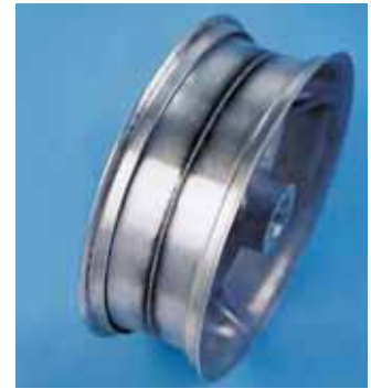
Fig. 76: Rim of a motorbike made of pressure diecast aluminium.
