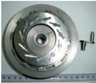
Fig. 60, 61: Control ring for turbo chargers. Front and reverse side with 11 circular EB welds.
