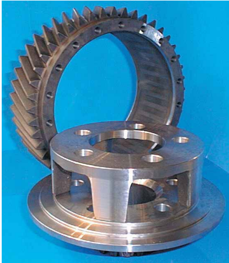
Fig. 124, 125: The triangular cross section of a truck planetary pignon cage has to be welded across the full profile.
