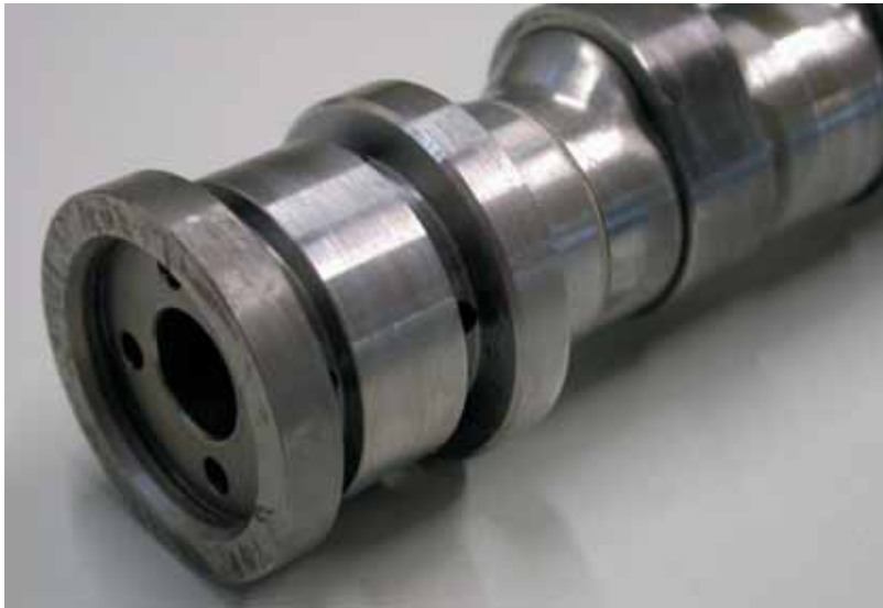
Fig. 36: Hollow camshaft with EB welded endpieces.
