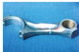
Fig. 43: Shortened piston rod.
