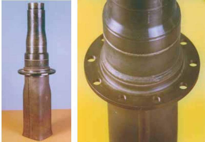
Fig. 73, 74: Stub shaft of a truck axle is welded to the axle (upper weld). The break-shoe carrier is EB welded with several weld runs to increase weld width.
