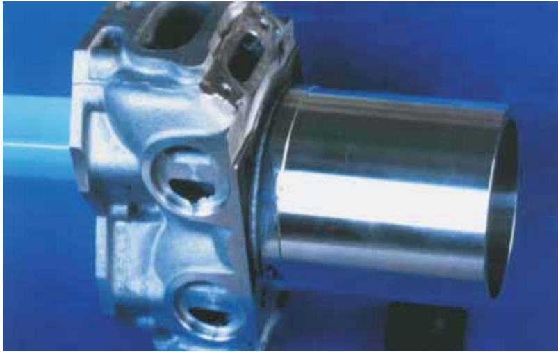
Fig. 28: Liner of hyper- eutectic aluminium alloy EB welded to dissimilar alloy with better stiffness.
