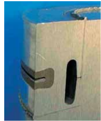
Fig. 29: Slender EB welds allow to produce a cooling channel without a lost core for casting.
