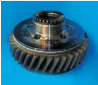
Fig. 124, 125: The triangular cross section of a truck planetary pignon cage has to be welded across the full profile.
