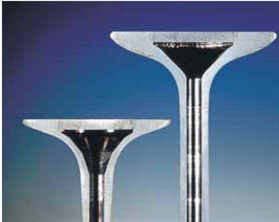
Fig. 44: Valves cooled by a heat pipe system.
