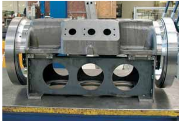
Fig. 195: Quill bearing boxes welded to the axel casting.
