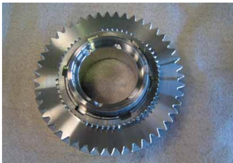
Fig. 102: The synchronizing ring with low mass and the gear with high mass warm up and expand at different speed. This is the typical weld situation when welding gears.
