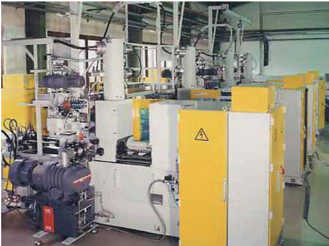
Fig. 35: Twin chamber machines for surface treatment of cams.
