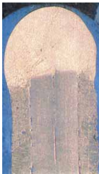
Fig. 65: Cross section through 4 layer edge weld of the particle filter.
