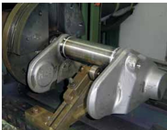
Fig. 224: Rocker arm for steering the boat in Fig. 225.
