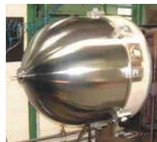
Fig. 169: Pole piece of a tank welded from outside.
