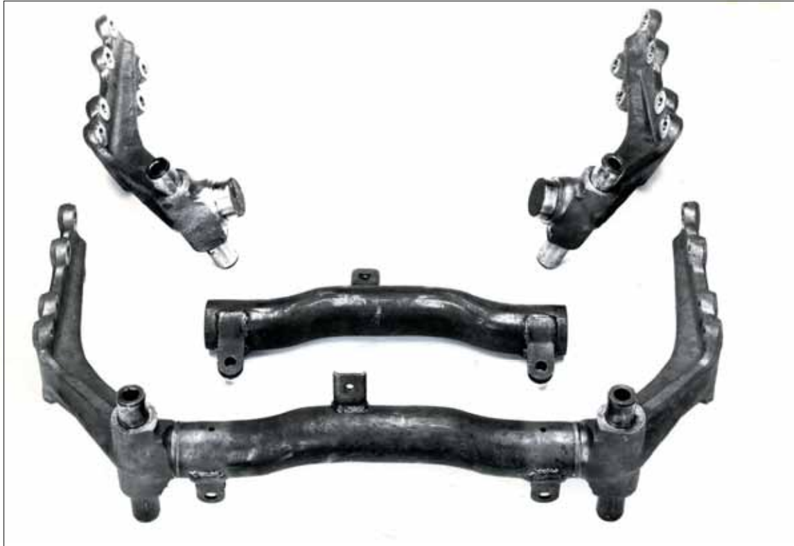
Fig. 75: SUV axle joined from 2 forgings and a preformed tube.
