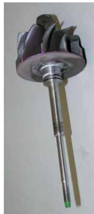
Fig. 56: Turbocharger: Impeller made from a superalloy, shaft of case hardening steel.
