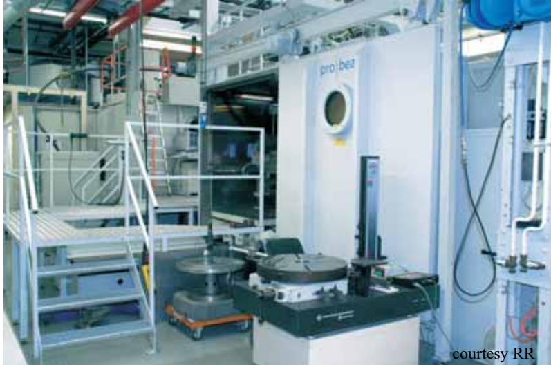
Fig. 148: EB welding machine for aircraft engine components with a 10 m 3 vacuum chamber, fully CNC controlled.
