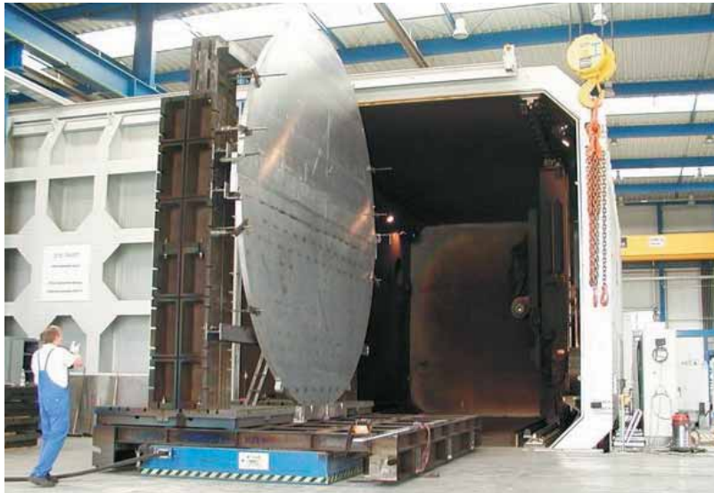
Fig. 177: The plate with 6m in diameter just fits into the vacuum chamber.
