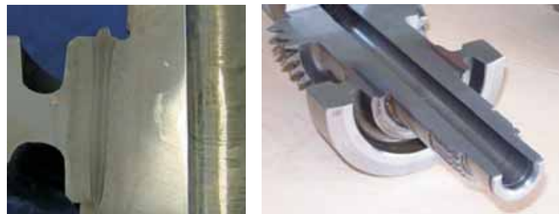
Fig. 135, 136: Cross section of drive shaft with 35 mm weld depth for high torque transmission. Weld position close to the shaft.
