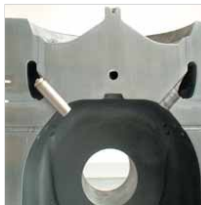
Fig. 31, 32: Pistons built from wrought and cast alloy make use of the design capability of EBW.
