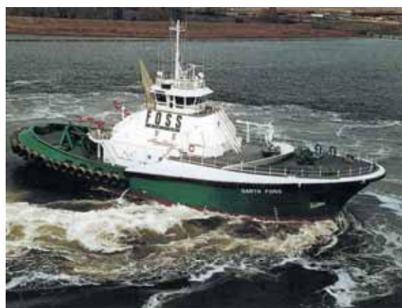
Fig. 225: A high tech propulsion system for tractor ships with variable thrust in power and direction allows to rotate the boat on the spot.
