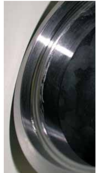
Fig. 85: Weld root at the suspension ring.
