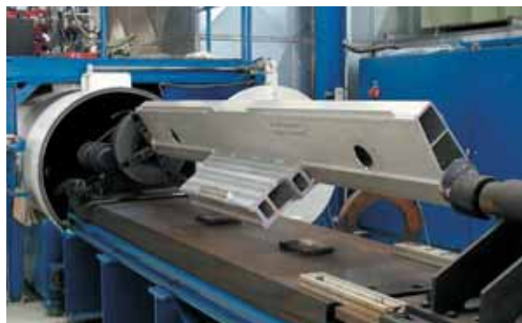
Fig. 188: Beamprofile with 2 EB welds, 35 resp. 40 mm penetration.
