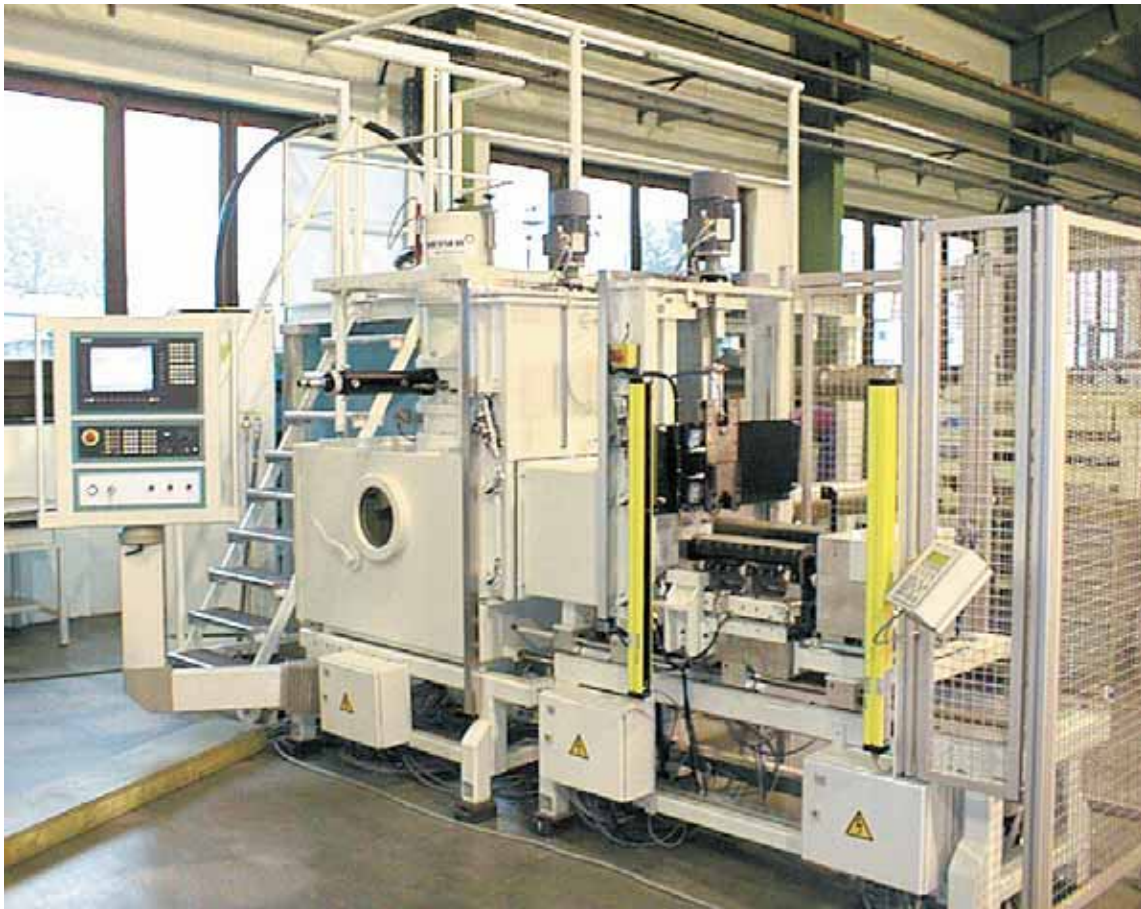
Fig. 1: High productive load-lock shuttle-machine for EB welding of pressure sensors. Automated loading and unloading with a gantry under clean room conditions.
