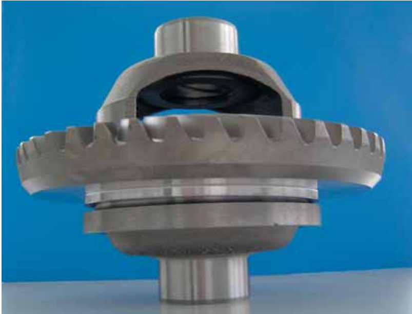
Fig. 68: Differential gear combines grey cast iron and case hardening steel.
