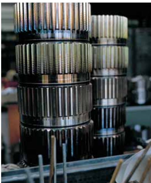
Fig. 115: Radial EB welds between flanges and gears.
