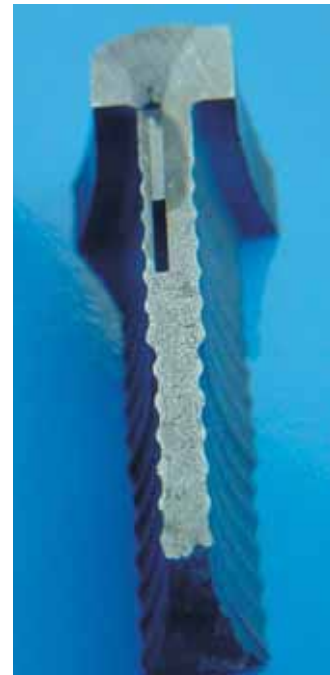
Fig. 15: The main welding problem results from offset of the slot due to large tolerances in the castings.
