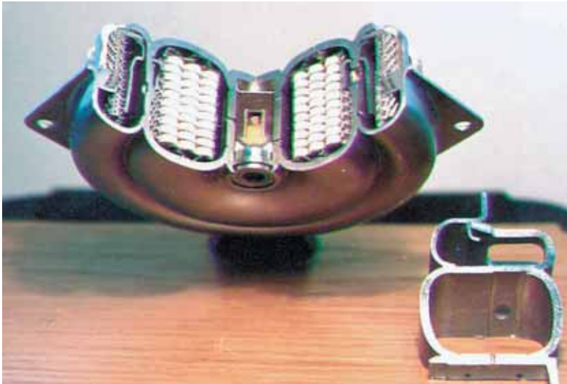
Fig. 89: Gas generators for driver airbags with 5 concentric EB welds.
