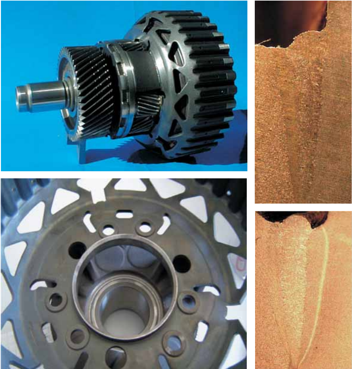
Fig. 128, 129, 130, 131: Planetary pignon cage with 3 radial welds (top) and drive gear, welded through the upper orifice. The part belongs to a CVT transmission.
