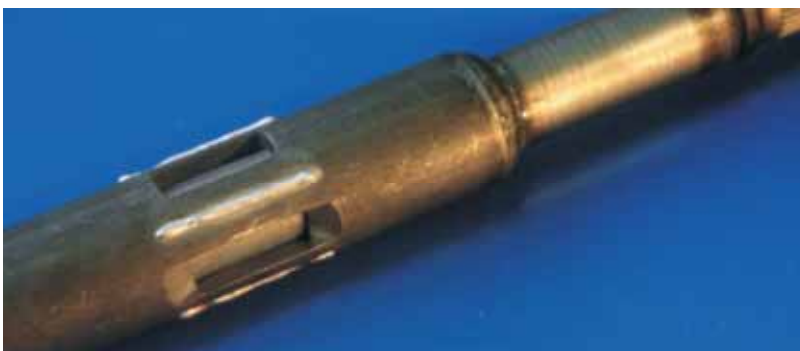
Fig. 86: Steering column with reinforcement for lock.
