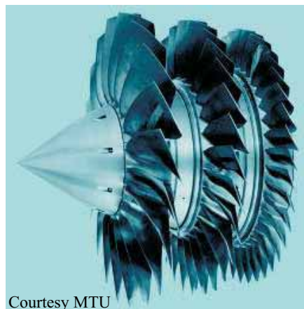
Fig. 151, 152: Blisks (bladed disks) are parts of the highest safety class. They are made of dissimilar Ti-alloys and used in the high pressure compressor. The blades are integral part of the disks. Circumferential welds join the disks to a rotor drum.
