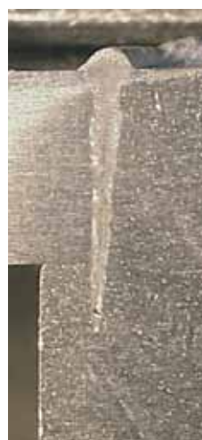
Fig. 57, 58: Valve head (flap) and related cross section of the weld.
