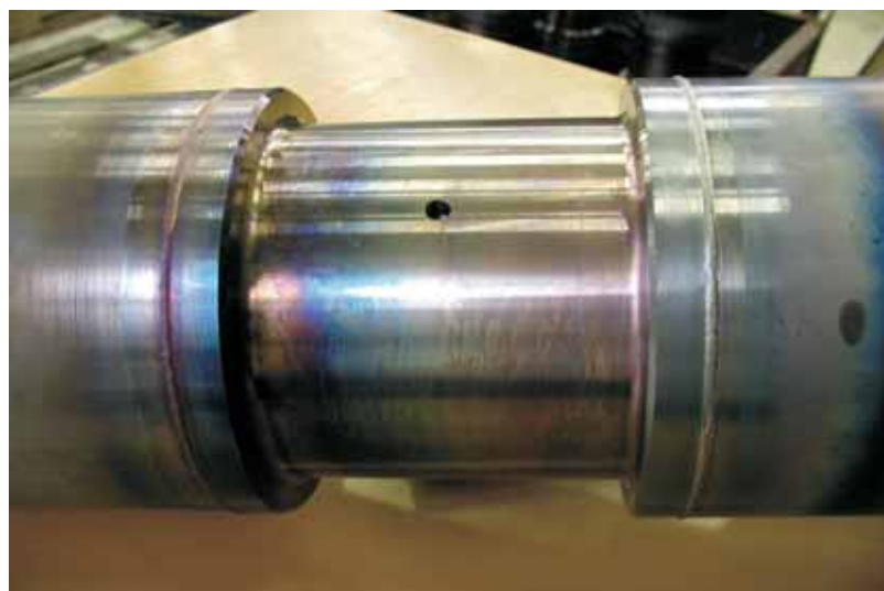
Fig. 198: Intermediate shaft with 2 welds.
