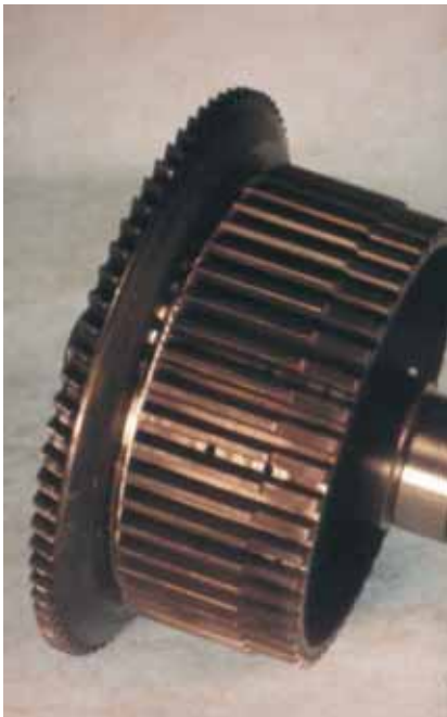
Fig. 113: Sintered clutch drum welded to a deformed gear disk and a shaft.
