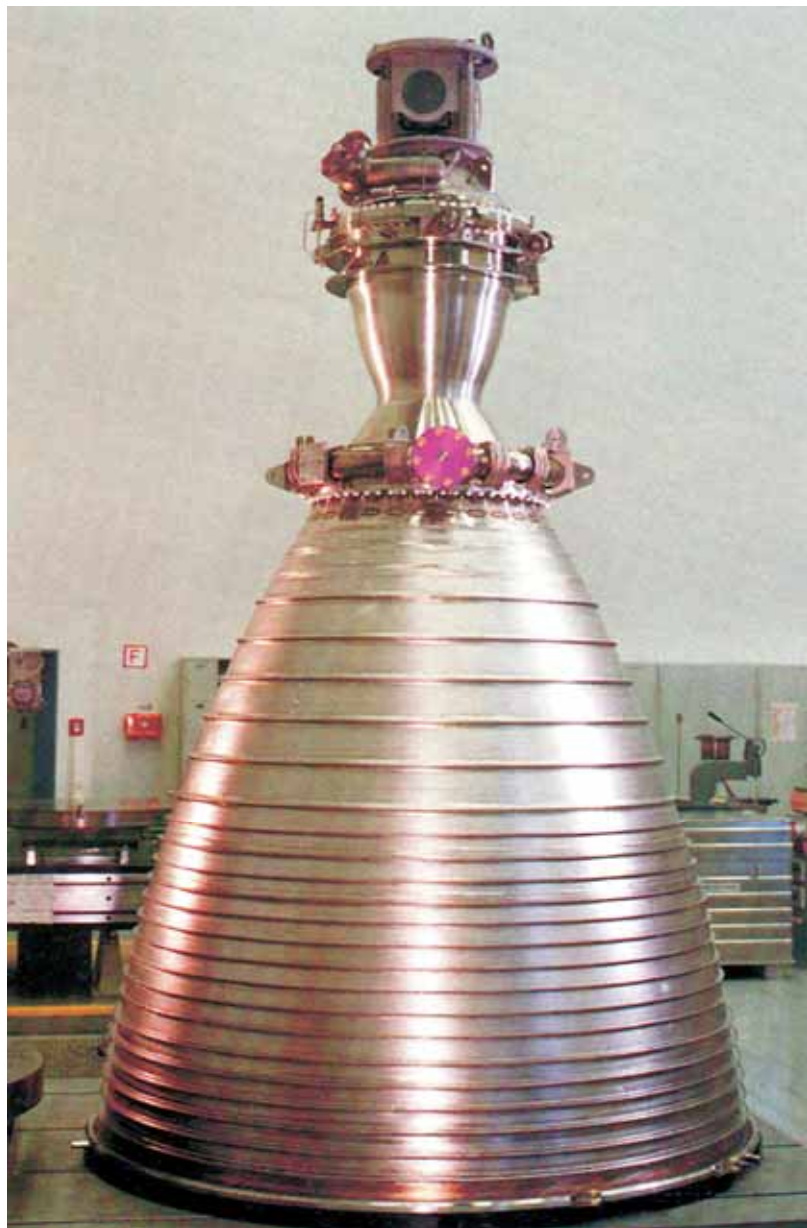
Fig. 180: Thrust nozzle for Ariane. The LOX-dome is located on top of the nozzle.
