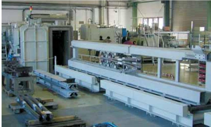
Fig. 212: The EB welding machine with clamping yoke.
