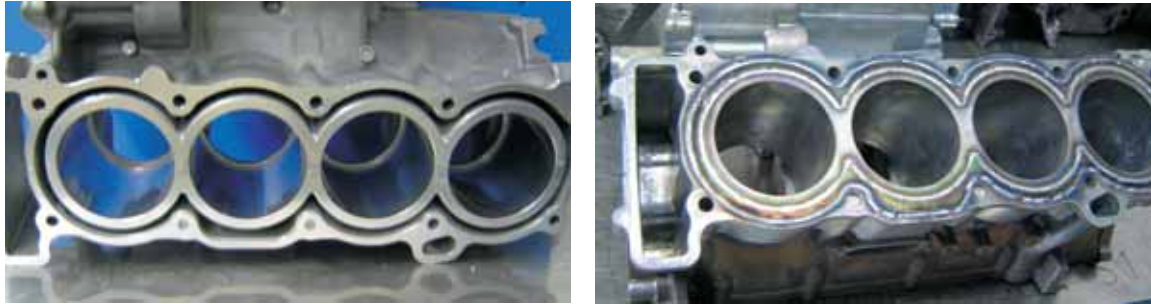
Fig. 17, 18: Closed deck motor blocks. Left: open; right: closed with contour welds.
