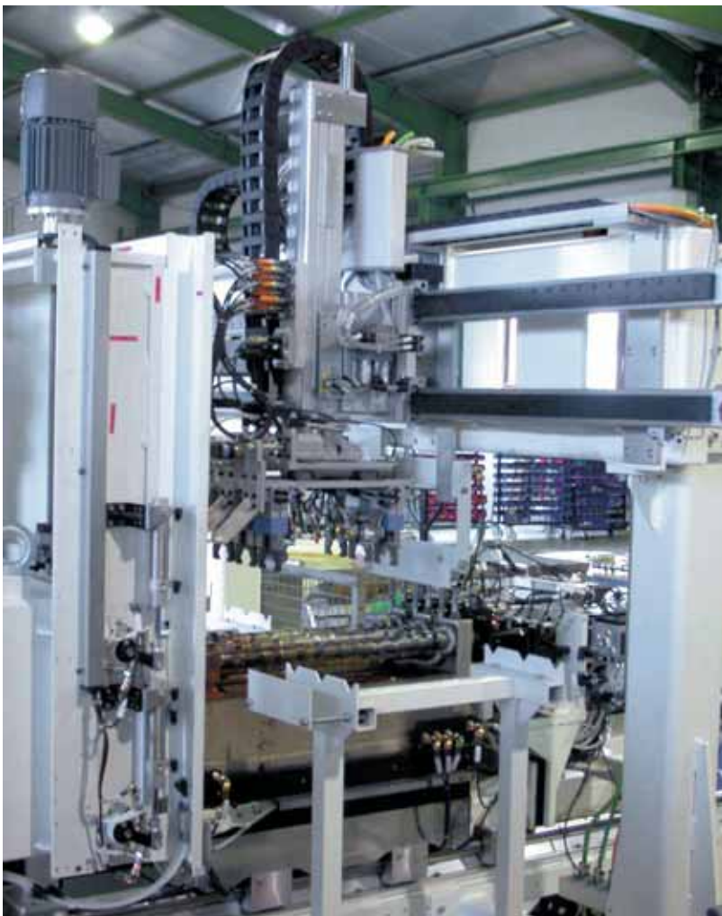
Fig. 37: Production line for EBW of camshafts with pre- and post- processes.
