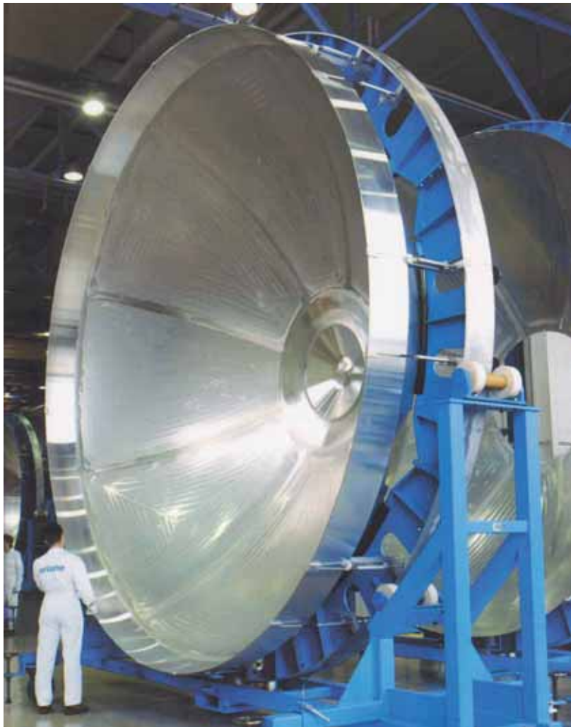
Fig. 173, 174: Ariane tanks for main (right) – and upper stage (above), forged from welded plates and machined.
