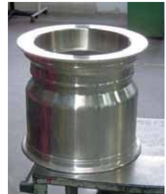
Fig. 77, 78, 79: Rims for race cars welded from forged magnesium alloys. Weld depth 20 mm.
