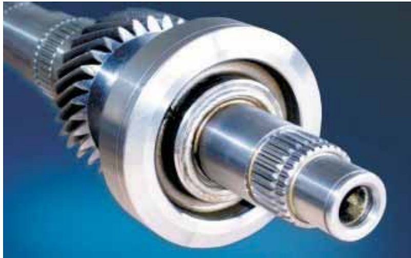
Fig. 66: Driveshaft of a SUV. The weld with 35 mm penetration has to carry a torque of 750 Nm (see fig. 135, 136).
