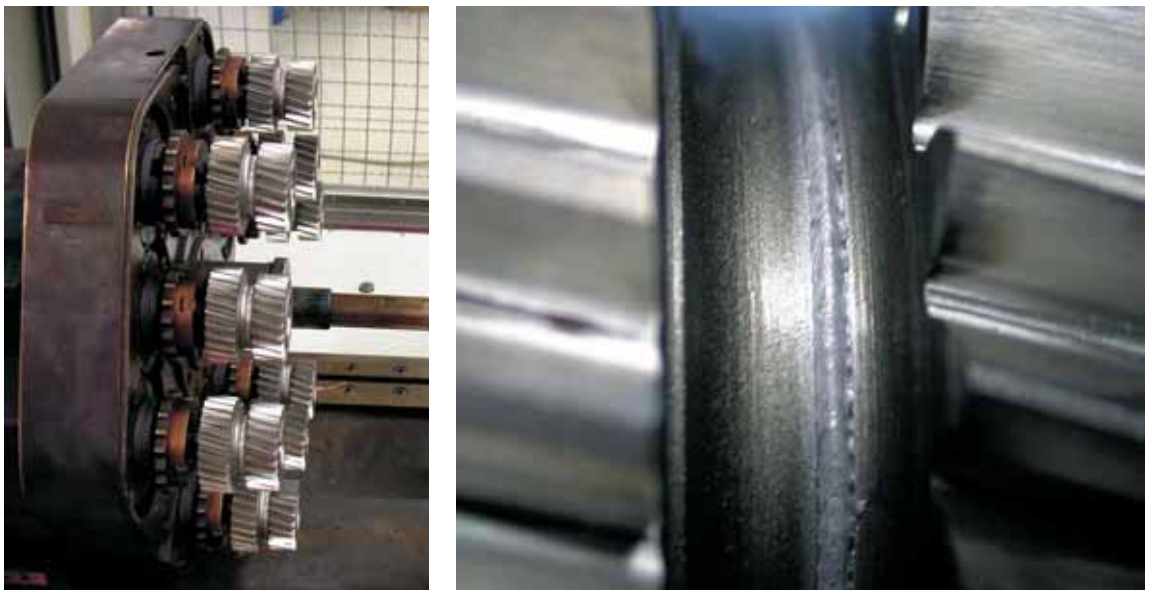
Fig. 122: Multi spindle unit for economic welding of gears on small volume production.
