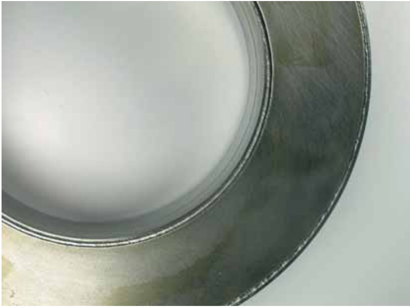
Fig. 40, 41: Viscous vibration damper, top view and cross section of the 2 welds of a differ- ent type.
