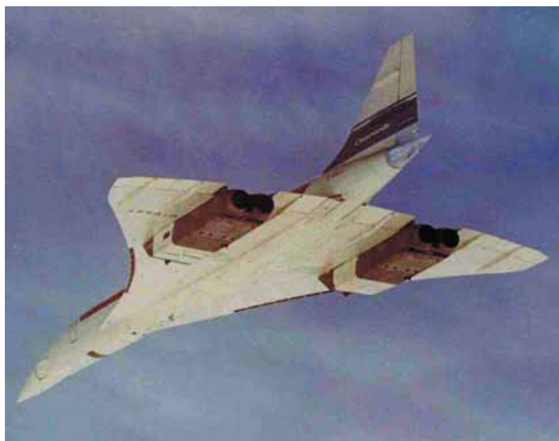
Fig. 140: The supersonic Concorde with the nacelle doors covering the engines.
