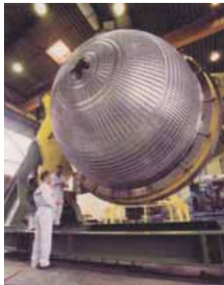
Fig. 173, 174: Ariane tanks for main (right) – and upper stage (above), forged from welded plates and machined.
