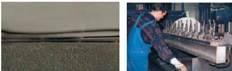
Fig. 200, 201, 202: The point of the switch is reinforced on its surface by wear-resistant maraging steel. Weld penetration 100 mm.
