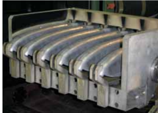
Fig. 144: Multiple tool for welding armrests from 4 sides.
