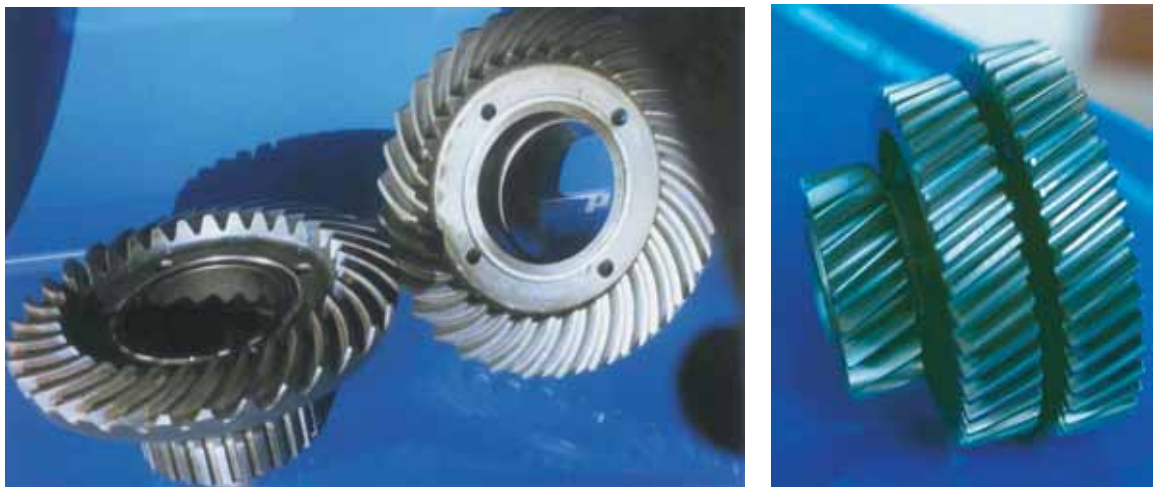
Fig. 111, 112: Bevel gears and triple gears are manufactured to advantage by machining each part individually. Subsequent joining requires a process with minimum heat input, as the parts are already hardened and minimum distortion to meet the tolerance specifications.
