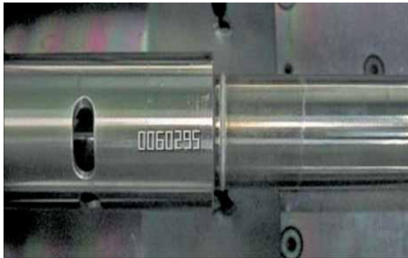
Fig. 81: Piston rod of a shock absorber with weld and identification by EB marking.
