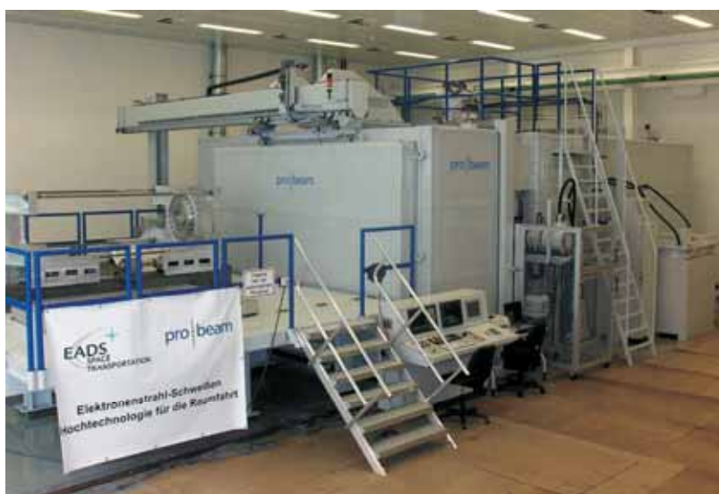
Fig. 170: Large EB welding equipment, special- ised for propellant tank welding with a vacuum chamber size of 45+10\text{m}^3 .
