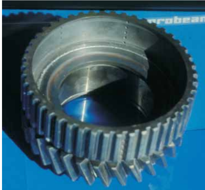
Fig. 114: Joining of forged and machined gear blanks.
