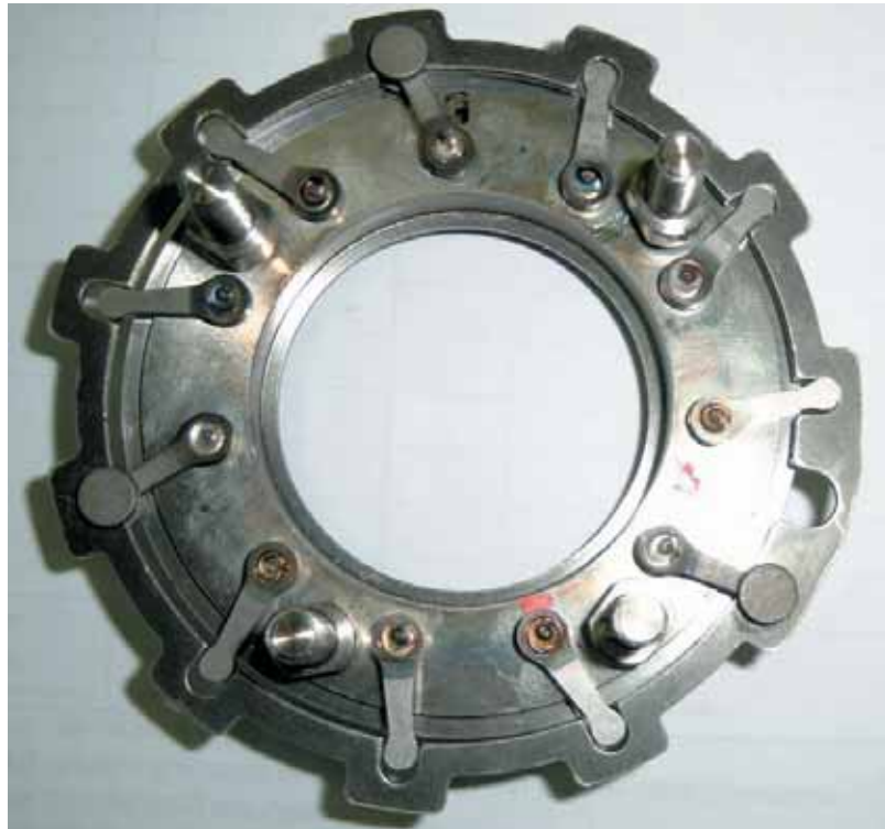
Fig. 60, 61: Control ring for turbo chargers. Front and reverse side with 11 circular EB welds.
