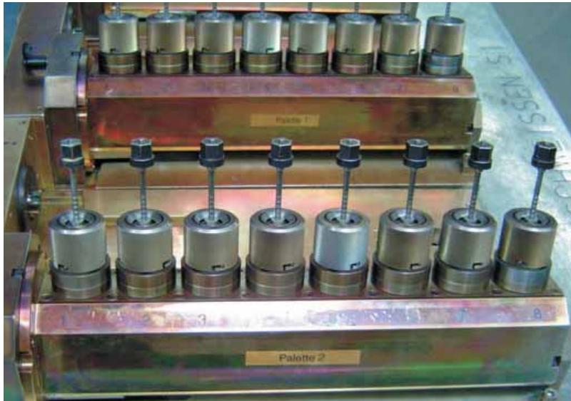
Fig. 53: Production tool for welding injectors.
