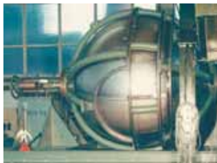
Fig. 167, 168: Old Ti-tank from 1965 with meridional welds.
