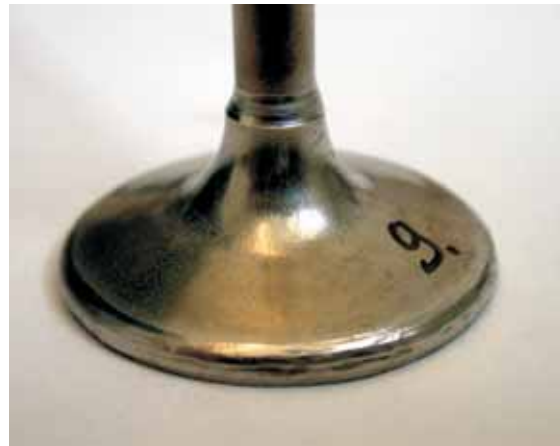
Fig. 45: Standard light-weight valve with hollow interior and fusion treated sealing edge.
