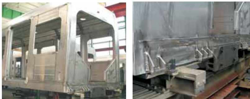
Fig. 186, 187: Railroad car with EB welded cross beam.
