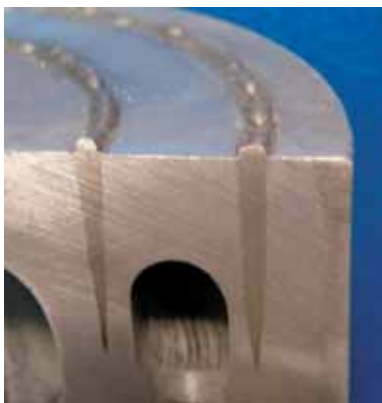
Fig. 30: The cooling channel on smaller pistons is welded with 2 parallel seams.
