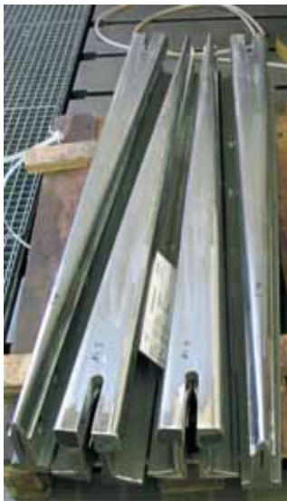
Fig. 213: 4 switch points for testing.
