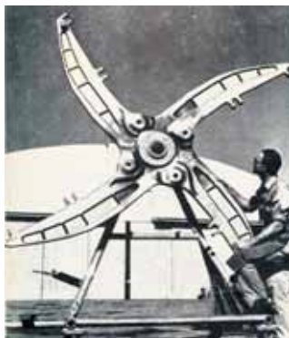
Fig. 138: A safety critical part is the assembly of four forged Titanium segments by 4 EB welds to a hub which carries the rotor blades of the Cheyenne helicopter.
