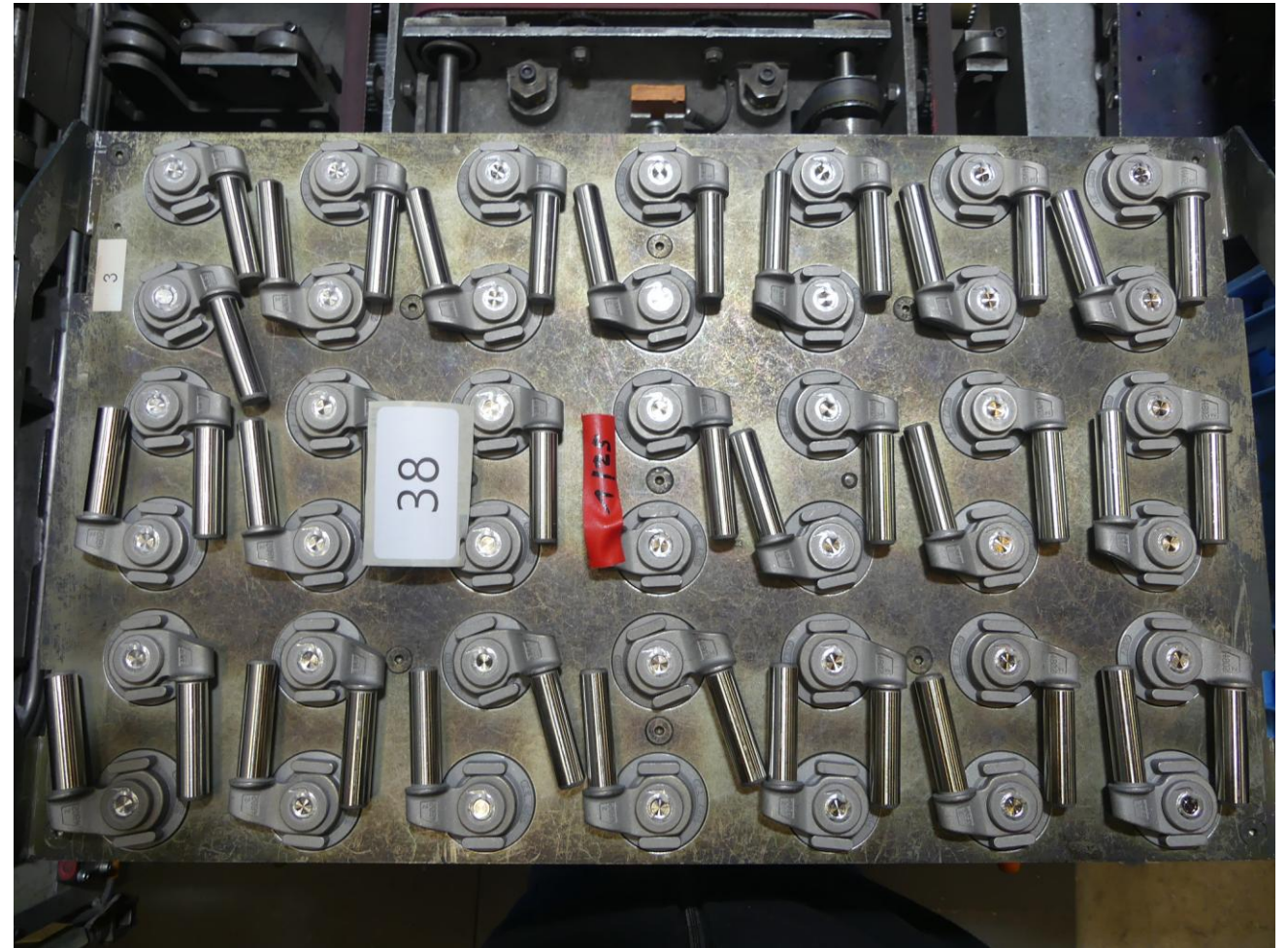
Fully charged palette after welding
