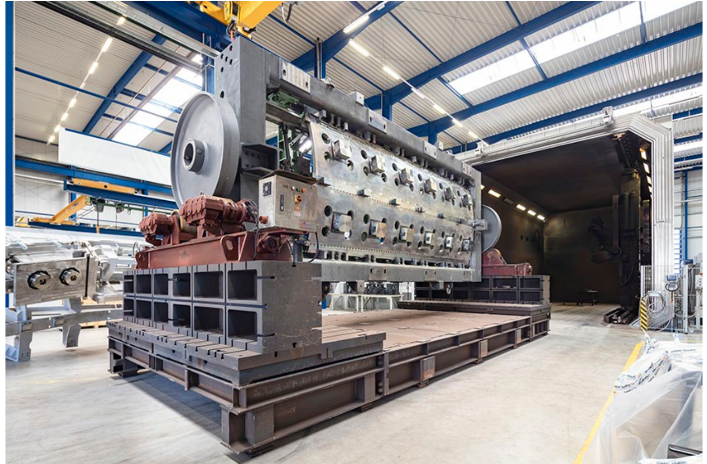
section of the ITER reactor vessel (80 t and 120 m weld length)
