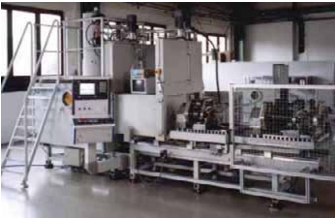
Fig. 120: EB shuttle machine with simultaneous welding, evacuating and loading.
