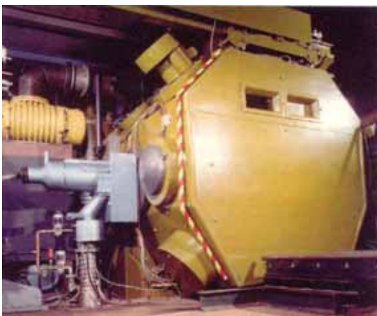
Fig. 103: TWI, EB welder 6m 3 chamber with 150 kV, 75 kW gun.
