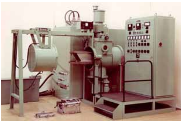
Fig. 75: Standard vacuum EB welder BW 700; 3 kW, 150 kV.
