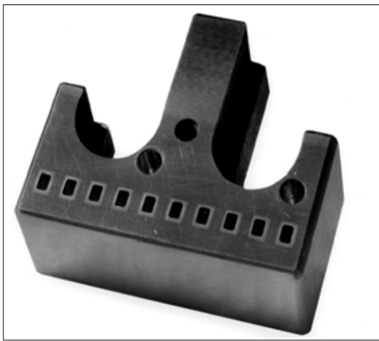
Fig. 25: Bottom die of a film cutting matrix EB transformation hardened.
