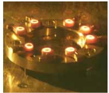
Fig. 126: EB flash welding of turbo-charger components.
