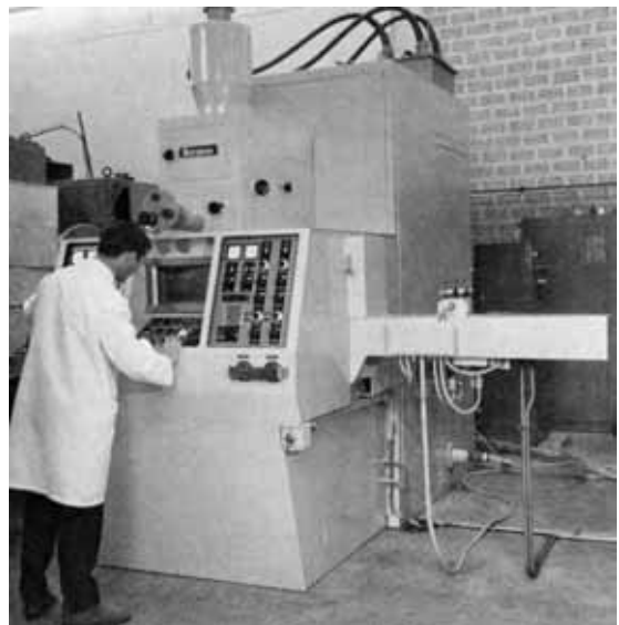
Fig. 77: Hard vacuum EB welder ESW 1000/3 for automatic production of print-hammers.
