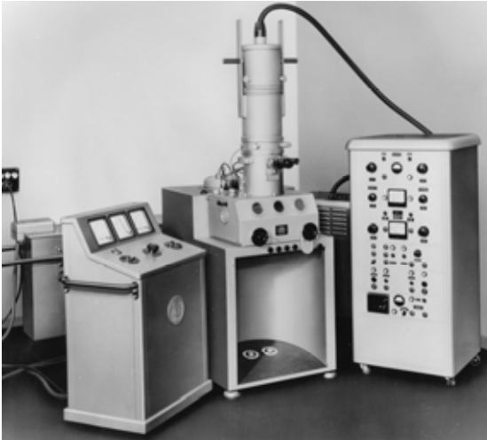
Fig. 48: 1960s-style Zeiss EB welder ES1002.
