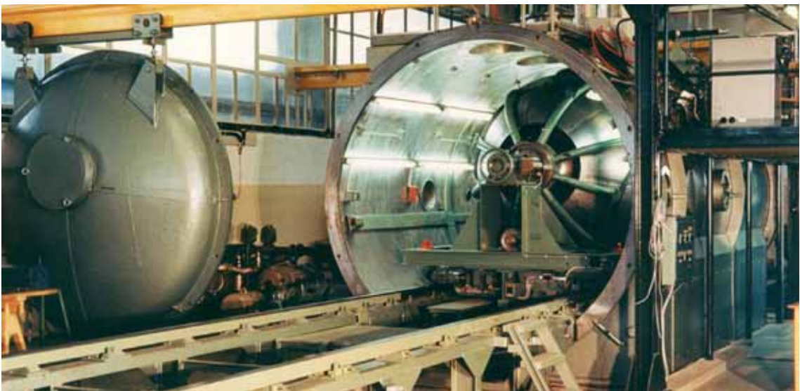
Fig. 18: The VFW machine for welding fuel tanks for the ELDO rocket (1965).
