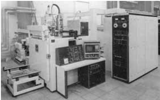
Fig. 86: Computerized EB welder with 15 kW, 60 kV (1984).
