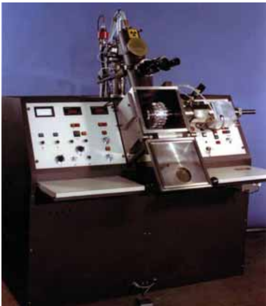
Fig. 111: Left: Wentgate desk-type machine, 1975, 50 kV, 2 kW.
