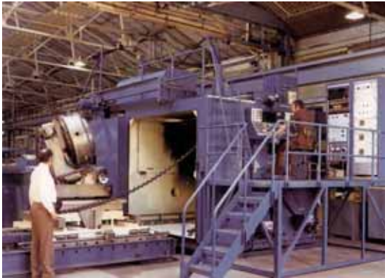
Fig. 105: Dynaweld machine with 3.5 m 3 vacuum chamber, 1967, 150 kV, 6 kW.
