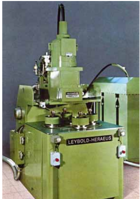
Fig. 79: Right: Partial vacuum EB welder for gear production.
