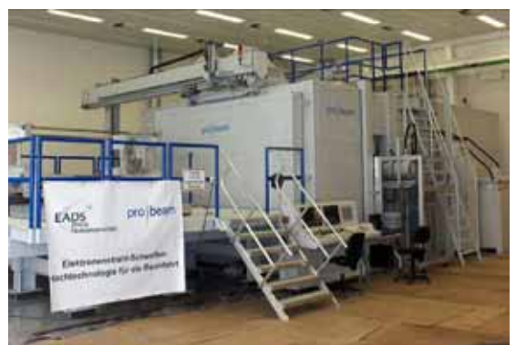
Fig. 123: 45 m 3 + 10m 3 chamber for welding of satellite tanks.
