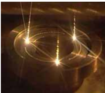
Fig. 124: 3 beam welding of gears.
