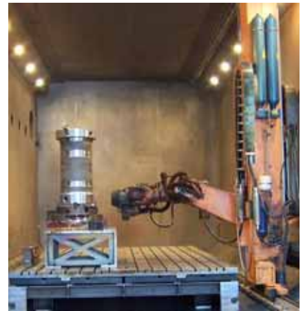
Fig. 129: High-voltage EB gun mounted on a robot.
