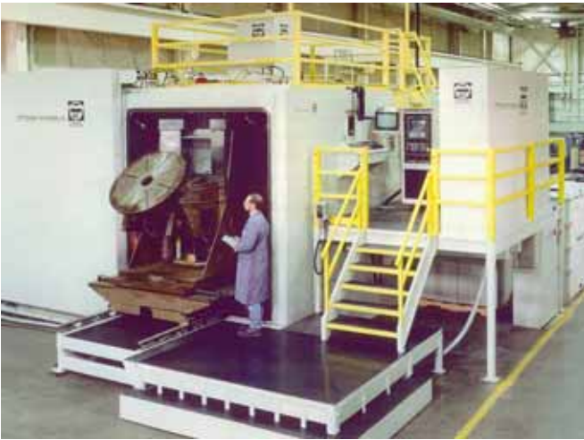
Fig. 59: Modern day, large chamber/fully CNC controlled version EBW unit made by PTR.
