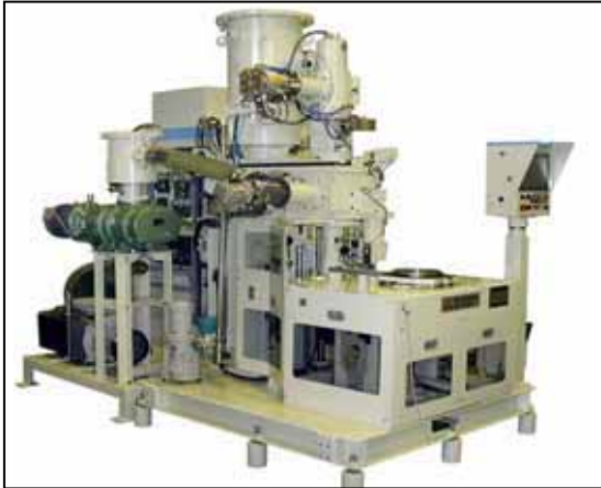
Fig. 95: A recent multi-stage EBW machine (MELCO).
