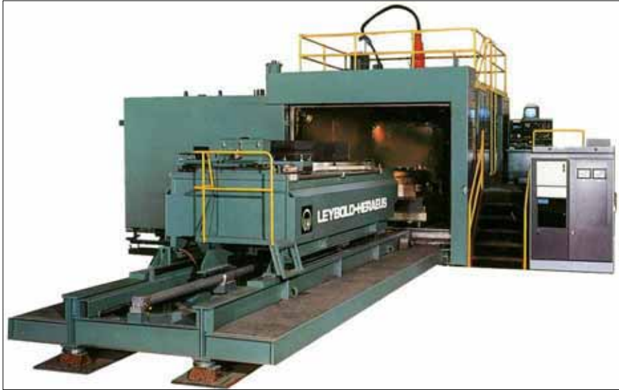
Fig. 89: EB welding machine EBW 3600/ 60-150 CNC for automated welding of steam turbines.
