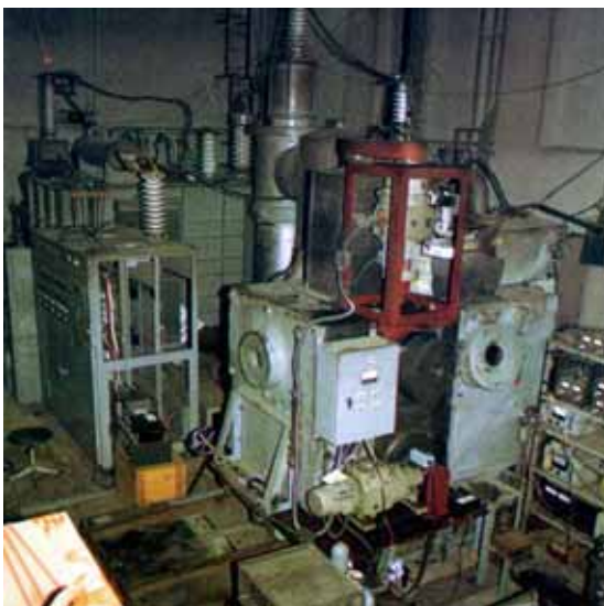
Fig. 91: The world's first EB welder 1972 with 100 kV, 100 kW continuous power output at Osaka University [66].
