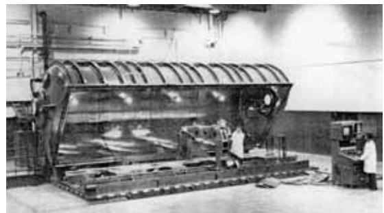
Fig. 55: 1970s version specialized EBW unit made by Sciaky called "clamshell".
