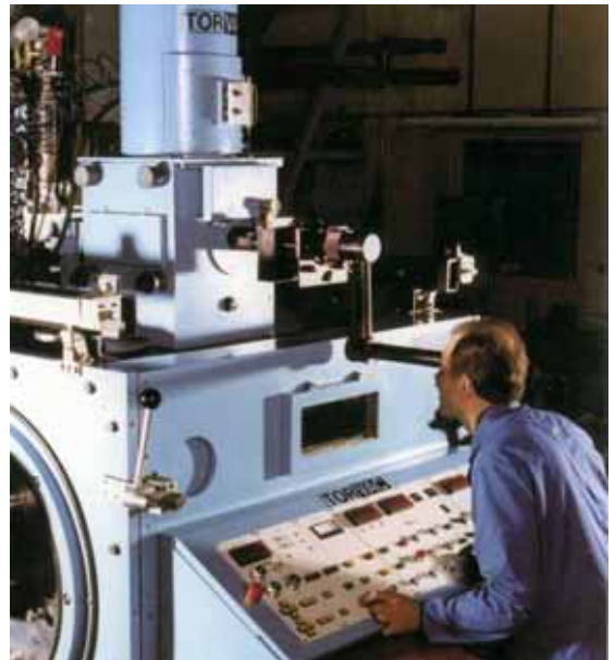
Fig. 110: Torvac machine with 1 m 3 chamber, 1984, 150 kV, 10 kW.
