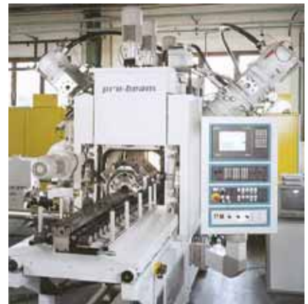
Fig. 121: EB transfer welder with pre- and post load-lock chambers and 2 EB guns.
