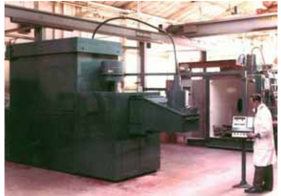
Fig. 106: Dynaweld, air to air, the tooling would be fitted under the nozzle, 1967/68, 150 kV.
