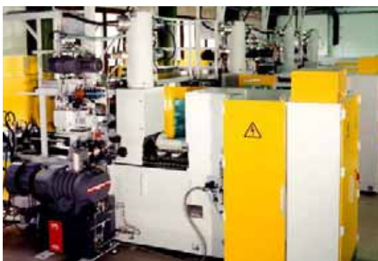
Fig. 122: Twin chamber machines for EB hardening of cam-shafts.
