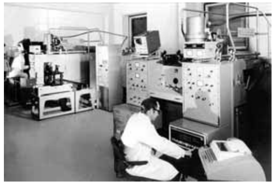
Fig. 20: Steigerwald EB machines, for micro-welding and drilling (1970) with CNC control for mechanical axes and beam parameters.
