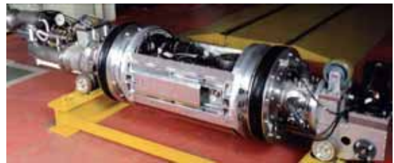
Fig. 98: Schematic diagram of a recently developed EBW machine for welding of high pressure gas pipelines in the field (above) and its realisation (KHI).
