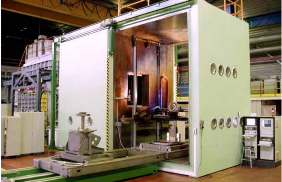
Fig. 69: General view of the typical vacuum chamber with box-shaped walls.
