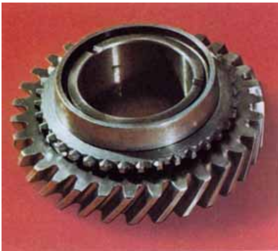
Fig. 78: Above: EB welding of synchronizing ring to gear.
