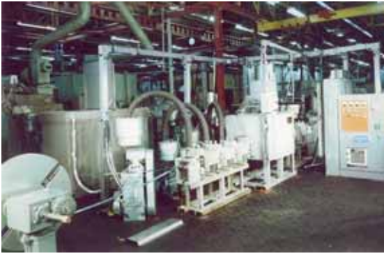
Fig. 44: Air-to-air style EBW system made by Hamilton Standard.
