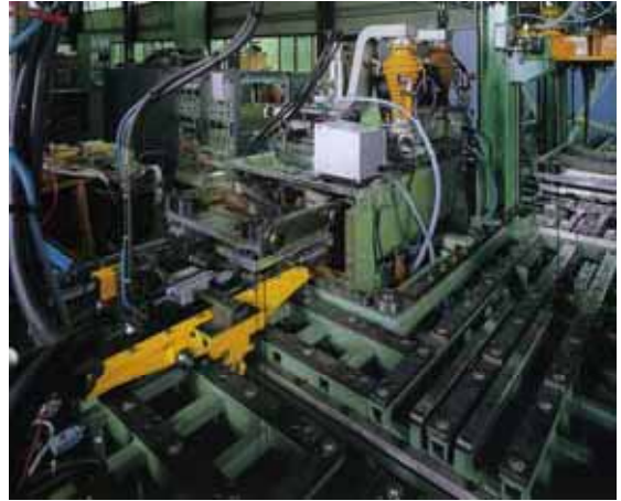
Fig. 42: Production machine for 500,000 parts per year manufactured by Techméta. The workpiece carriers are transferred around the chamber.
