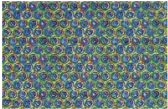
Fig. 24: EB texturing of steel rolls at Sidmar (2000).
