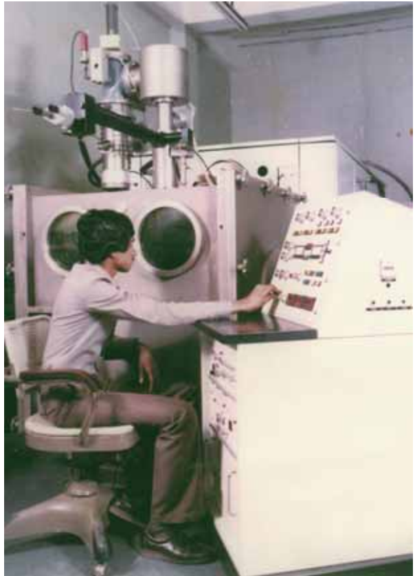
Fig. 108: Torvac machine with two chambers, 1978, 60 kV, 8 kW.
