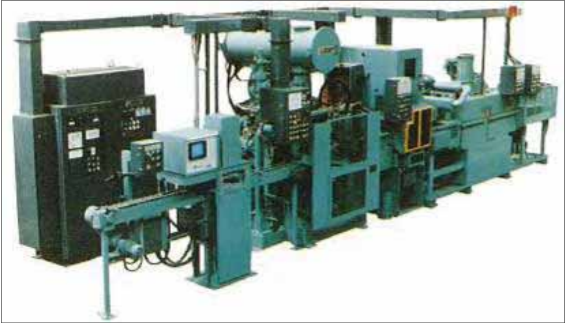
Fig. 93: The 1st EBW machine designed and produced by JEOL, which was adapted to soft vacuum (1959).
