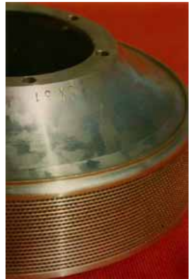
Fig. 22: EB drilled fiberizer for glass wool production.
