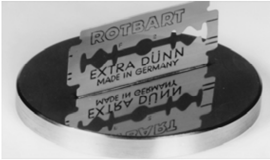
Fig. 11: EB welding of thin to thick was remarkable in the late 1950s.
