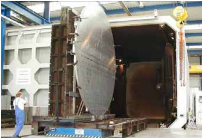
Fig. 128: 630 m 3 chamber with EB welded disc for Ariane tank.
