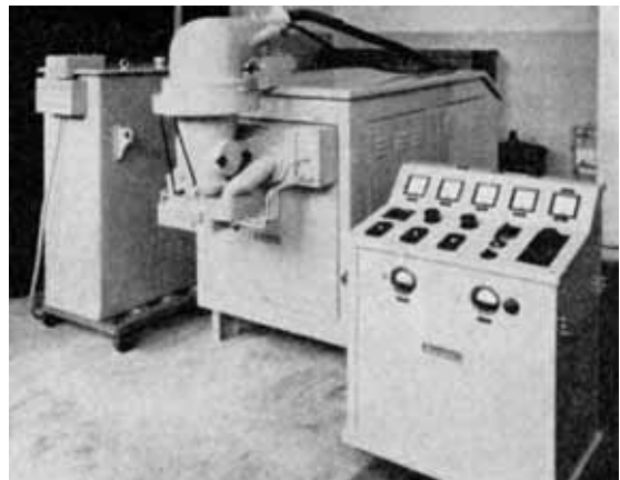
Fig. 74: EB equipment at W.C. Heraeus to weld on atmosphere, 3 kW, 160 kV.
