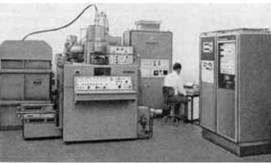
Fig. 82: Numerically controlled EB welder for hard and soft vacuum use.
