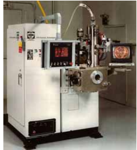
Fig. 60: Modern day, small chamber/PLC controlled version EBW unit made by PTR.
