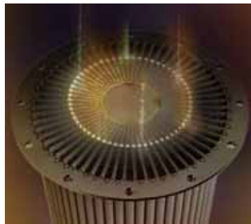
Fig. 125: 60 beam welding of particle filters.
