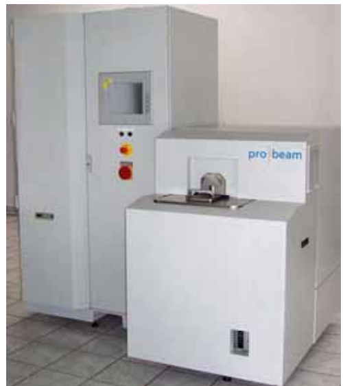
Fig. 119: Load lock cycle machine for rapid EBW of small parts in hard vacuum.
