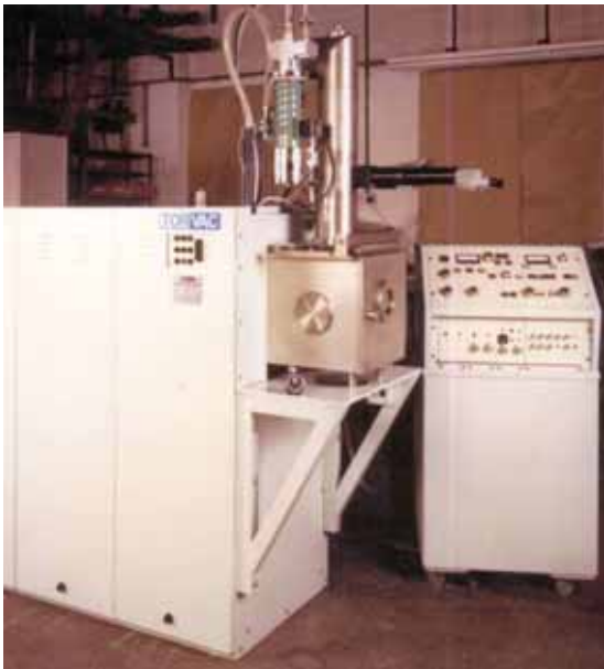
Fig. 109: Torvac general-purpose machine, 1974, 60 kV, 3 kW.
