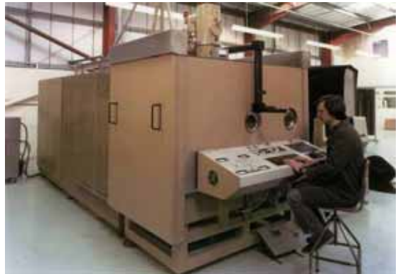
Fig. 111: Left: Wentgate desk-type machine, 1975, 50 kV, 2 kW.
