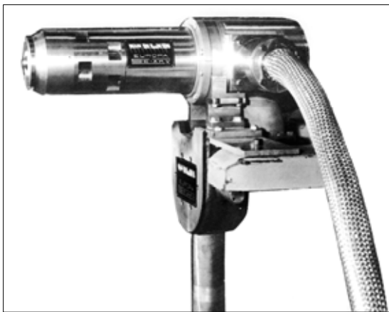
Fig. 38: EB gun for welding tubes into heat exchanger plates using local vacuum.
